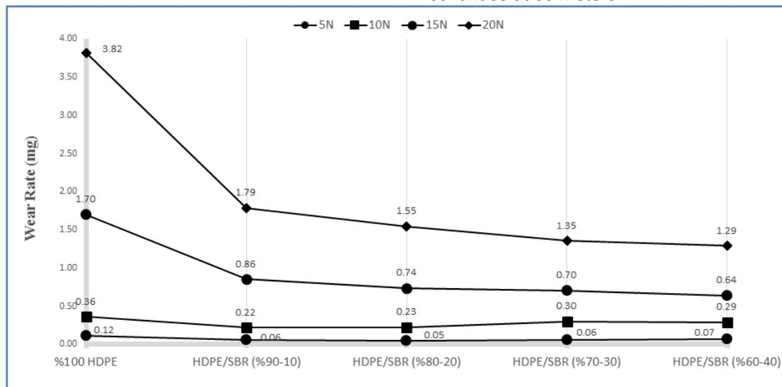
Fig. 2 - Applied load-wear loss relationship of HDPE polymer composites (Newton).
