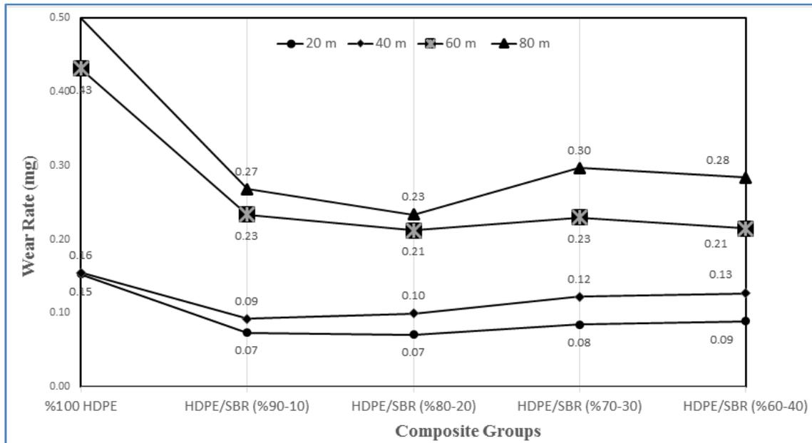
Fig. 1- Effect of sliding distance (meter).
