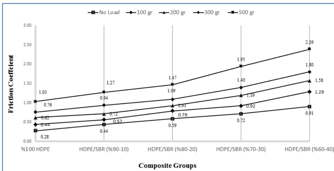
Fig. 3 - Friction values of HDPE and its composites.
