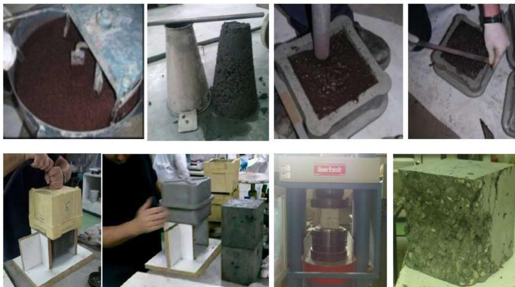
Fig. 9 - Procedure of preparation and testing of concrete cubes (EN 12390-3: 2003)
