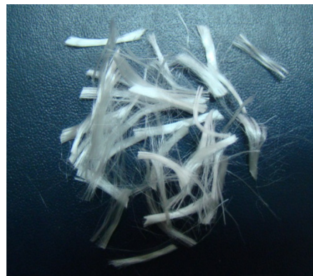
Fig. 3 - Eșantion de fibre polipropilenice / Sample of polypropylene fibres .
