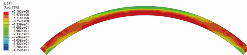
Fig.11 - The distribution of the stress from S11 vertical section of 2# test block.
