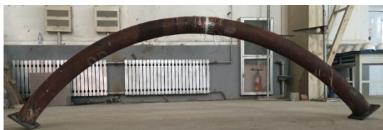
Fig.4 - Overall deformation of circular arch with 0.26 rise-span ratio.
