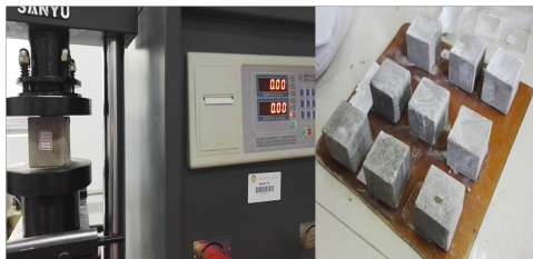
Fig. 16 - Uniaxial compressive strength and splitting tensile strength test.
