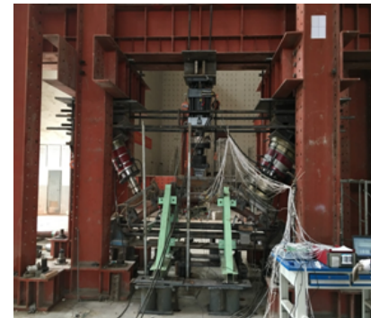
Fig.2 - The test bench and the pre-buried strain.
