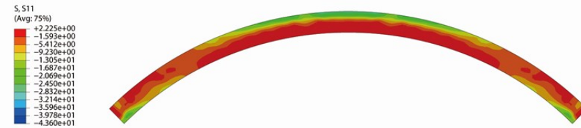
Fig.12 - The distribution of the stress from S11 vertical section of 3# test block.
