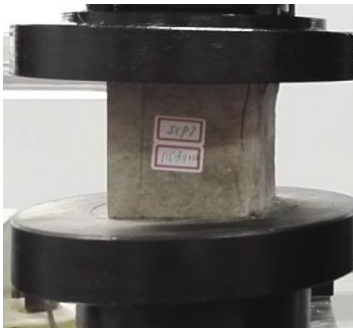
(a) Expansion of core concrete after elastic-plastic stage U, U3
