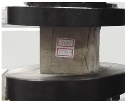
(a) Expansion of core concrete after destruction stage U, U3
