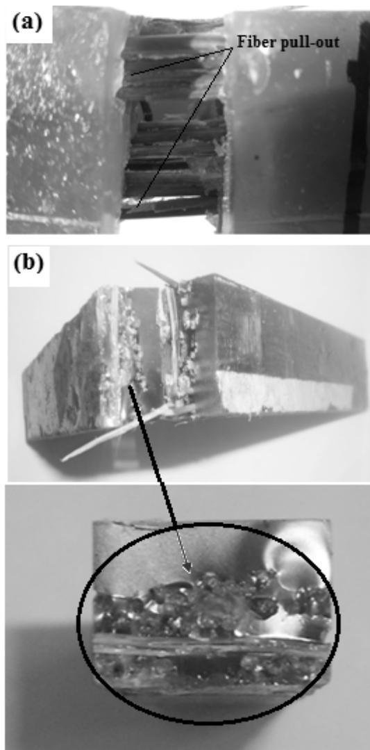
Fig.9 - Optical micrographs of the tensile fracture surfaces of (a) untreated woven Alfa fiber composite and (b) permanganate treated woven Alfa fiber composite.
