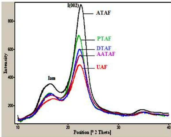
Fig.4 - X-ray diffraction patterns of untreated and treated Alfa fibers.
