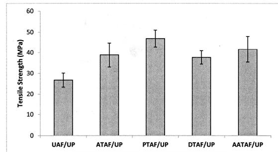
Fig.5 - Effect of fiber modification on tensile strength of woven Alfa fiber-unsaturated polyester composite.
