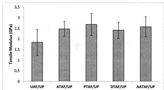
Fig.6- Effect of fiber modification on modulus strength of woven Alfa fiber-unsaturated polyester composite.
