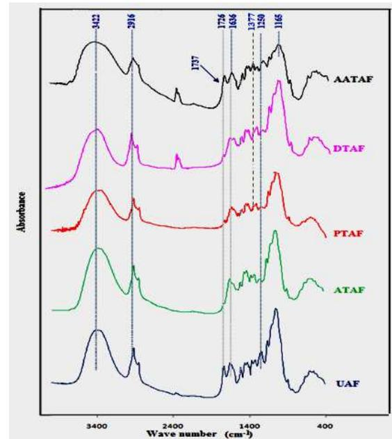
Fig. 2 - FTIR Spectra of the treated and untreated Alfa fibers.
