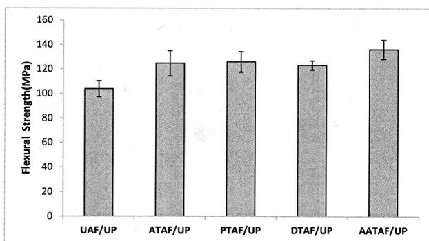
Fig.7- Effect of fiber modification on flexural strength of woven Alfa fiber–unsaturated polyester composite.
