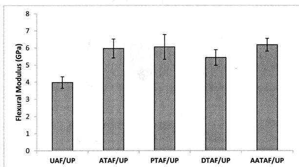
Fig.8 - Effect of fiber modification on flexural modulus of woven Alfa fiber–unsaturated polyester composite.
