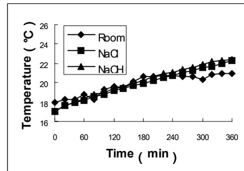
Fig.14 - Trend of solution temperature during the test (W/B=0.25,28 d).
