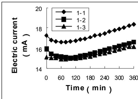
Fig.11 - Instantaneous electric current during the test (W/B=0.25, 28 d).
