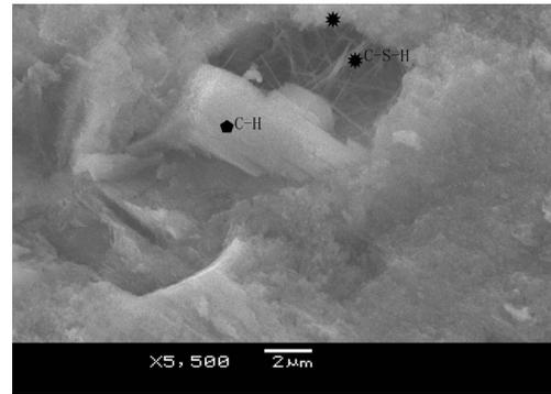
Fig.15 1-1 Paste SEM morphology(3d,W/B=0.25).
