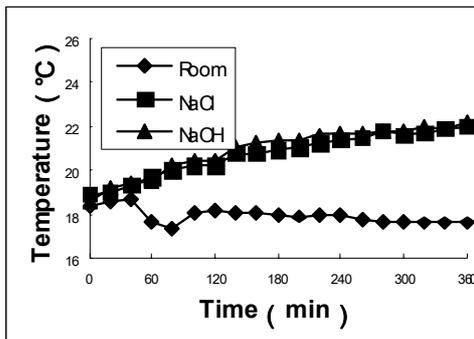
Fig.16 - Trend of solution temperature during the test (W/B=0.34,28 d).
