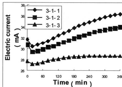
Fig.13 - Instantaneous electric current during the test (W/B=0.34, 28 d).
