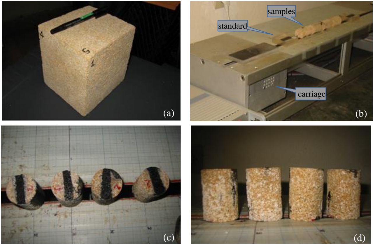
Fig. 3 – (a) Calcarenite block used for coring eight identical cylindrical samples: (c) four cores taken parallelly to the sediment bedding (series 1) and (d) four other perpendicularly to this one (series 2). (b) Four calcarenite cores between two standard samples positioned along the scanning direction on the platform of thermal conductivity scanner (TCS). The pictures (c) and (d) are taken after the first dissolution-crystallization cycle, and show the NaCl efflorescence formation.
