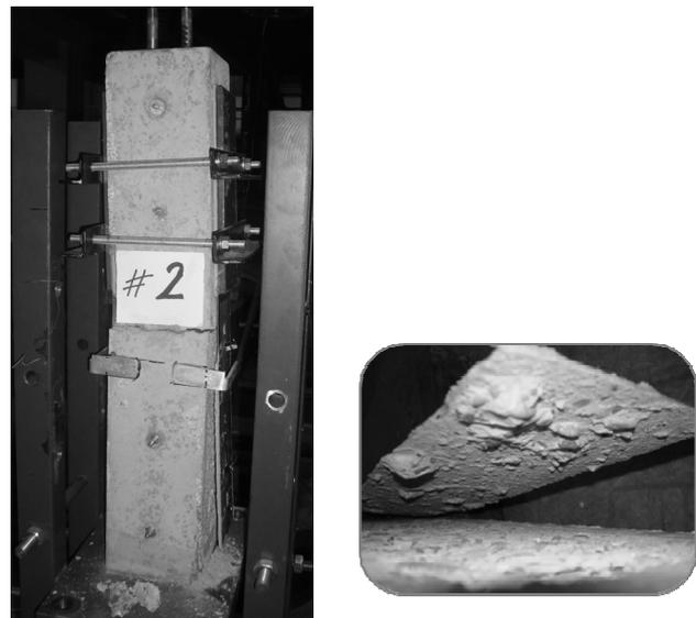
Fig. 6. Typical failure mode with a separation of a thin concrete layer
