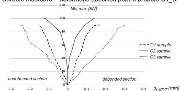
Fig. 9. The load slip curves
