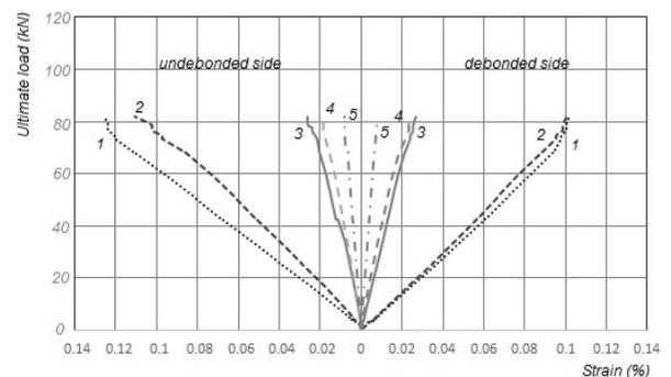
Fig. 8. The load strain curves for C1\_3 specimen
