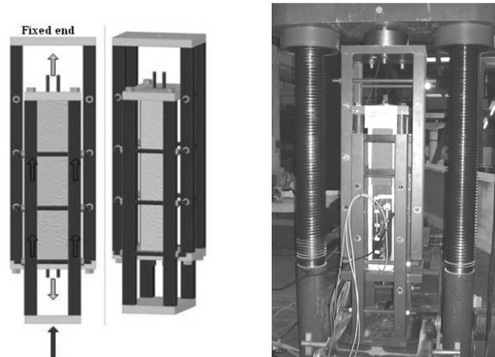
Fig. 4. The author's device utilized to apply the load on the specimens
