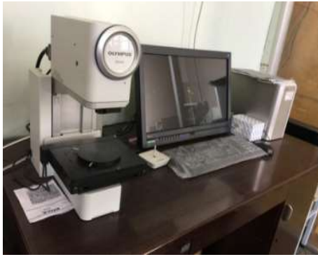
Fig. 1 - DSX-HRSU microscope with super depth of field.
