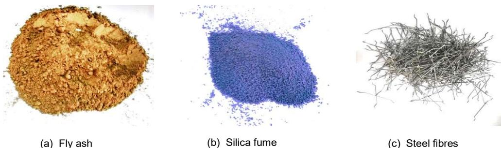
Fig. 1 - Diagrammatic representation of fly ash (a), silica fume (b) and steel fibres (c) used in the concrete mix.
