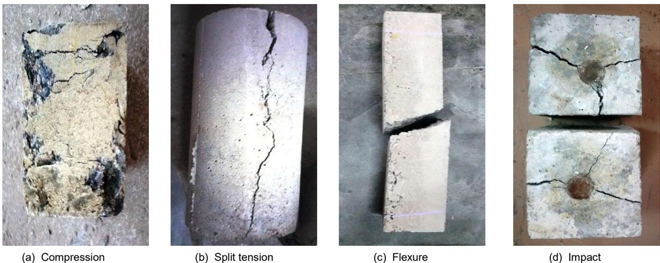
Fig. 2 - Failure of concrete in compression (a), split tension (b), flexure (c) and impact (d).
