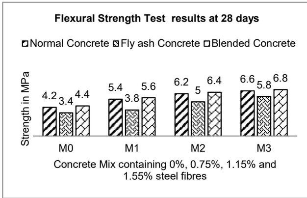
Fig. 5 - Flexural strength at 28 days
