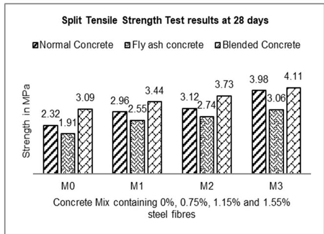
Fig. 4 - Split Tensile Strength at 28 days.
