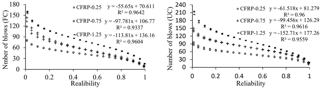
Fig. 3 - Scatter diagram of impact strength with fitted regression line.
