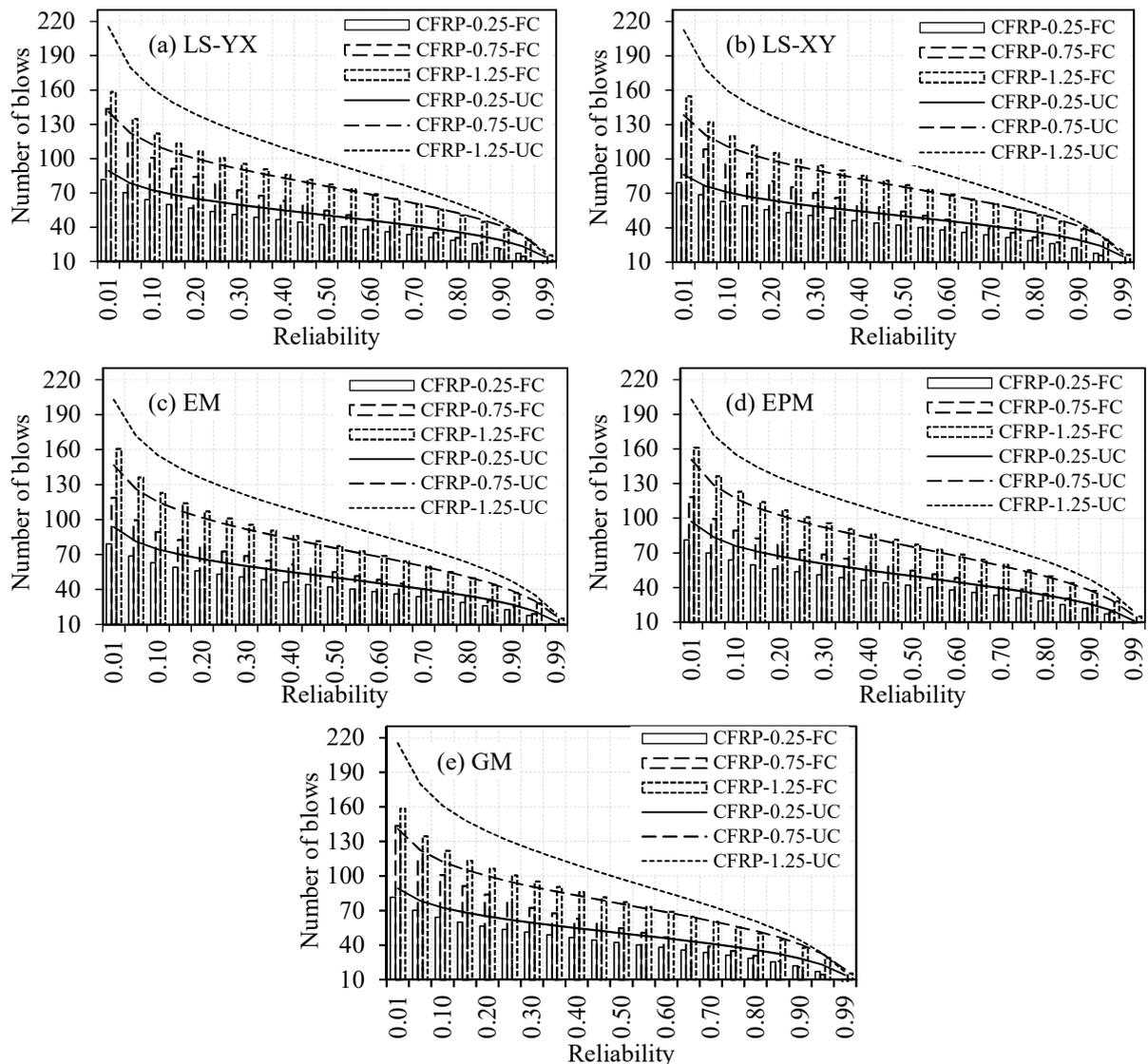
Fig. 2 - Impact strength (FC and UC) interms of reliability of different methods.
