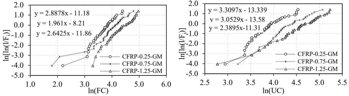
Fig. 1- Weibull lines from graphical method.
