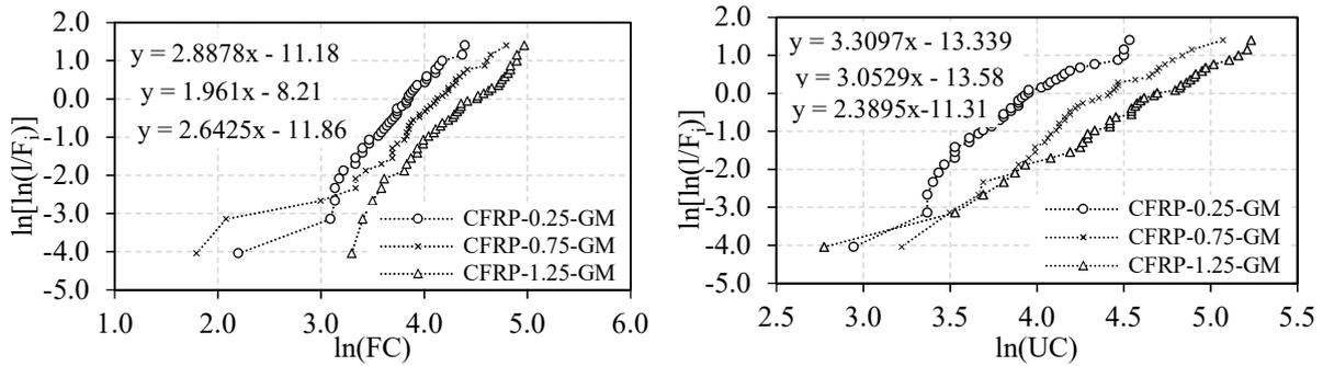
Fig. 1- Weibull lines from graphical method.
