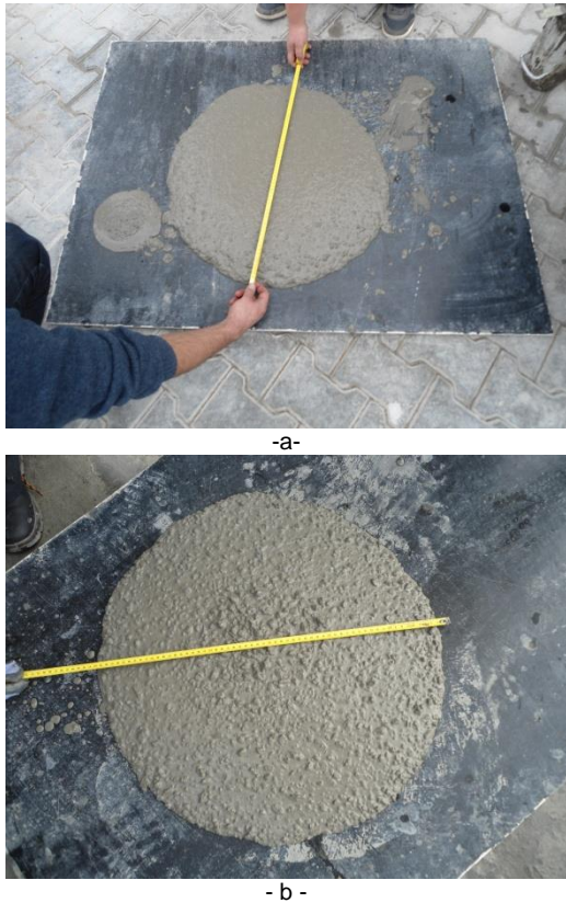
Fig. 4 - Slump-flow test of the reference concrete (NAC) – a and of RAC 100 – b.
