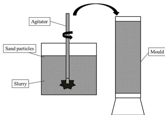
Fig. 1 - Schematic diagram of mixing process.
