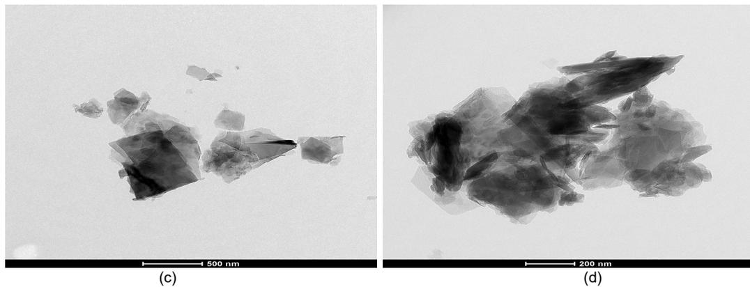
Fig. 7 -SEM images (a and b) and TEM images (c and d) of the bio-sandstones cemented by mixing process.
