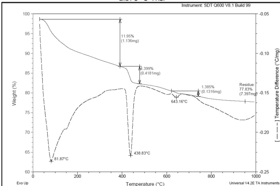
Fig. 7- TGA-DTA curves for a steam cured paste produced with Portland cement (100 CP).
