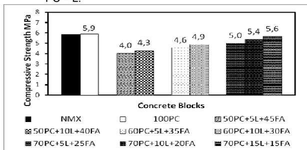
Fig. 3 - Compressive strength of concrete blocks cured with steam for specimens reference and ternary system PC – L – FA.
