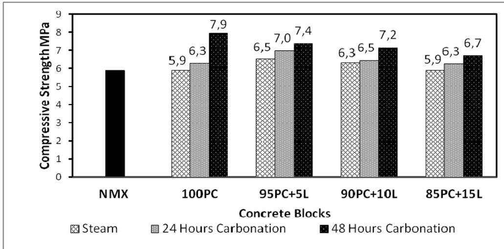
Fig. 5 - Compression strength of concrete blocks cured with CO<sub>2</sub> for specimens reference and binary system PC – L.
