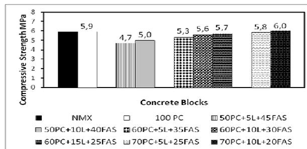
Fig. 4 - Compression strength of concrete blocks cured with steam for specimens reference and ternary system PC – L – FAS.
