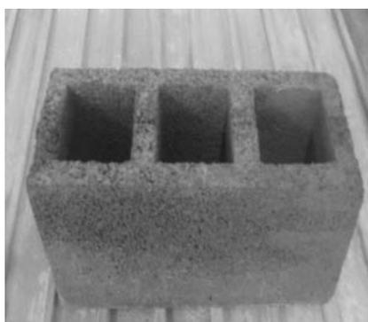
Fig. 1 - Concrete block (masonry unit) used to evaluate the properties targeted in this research.
