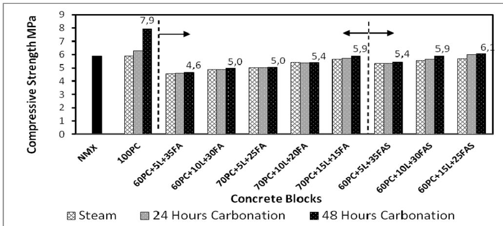
Fig. 6 - Compression strength of concrete blocks cured with CO<sub>2</sub> for specimens reference and ternary system PC – L – FA and PC – L – FAS.
