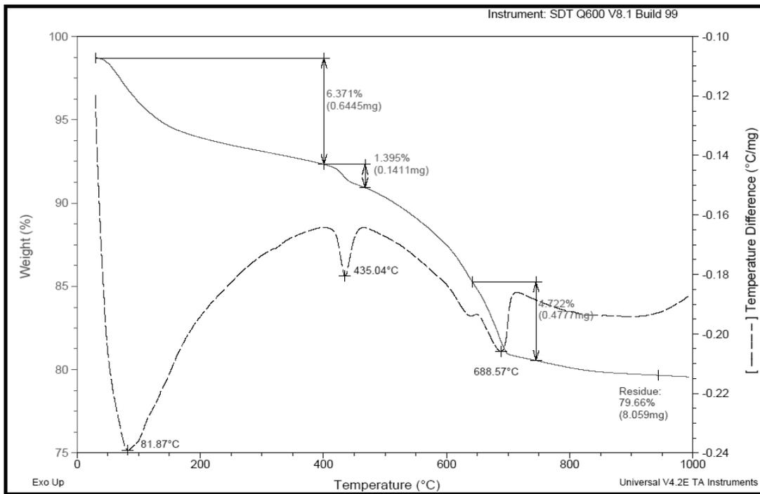
Fig. 8 - TGA-DTA curves for a 24 hour CO<sub>2</sub> cured paste produced with Portland cement (100 CP).
