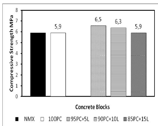
Fig. 2 - Compressive strength of concrete blocks cured with steam for specimens reference and binary system PC – L.
