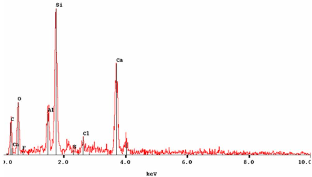
Fig. 4 - b) EDX analysis after GFRP pyrolysis / Analiza EDX după piroliza GFRP.
