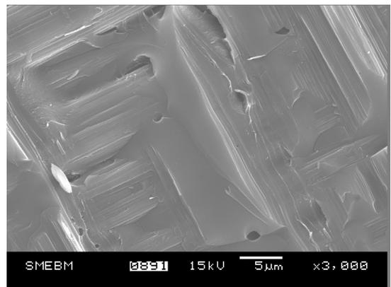
Fig. 8. - a) SEM analysis after CFRP pyrolysis/ Analiza SEM după piroliza CFRP
