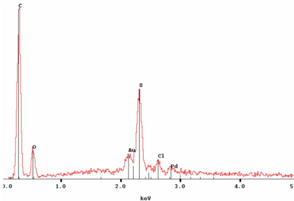
Fig. 8 - b) EDX analysis after CFRP pyrolysis / Analiza EDX după piroliza CFRP.
