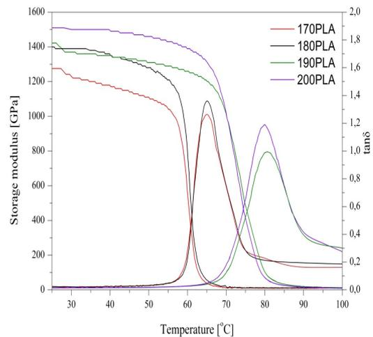
Fig. 3 - DMTA curves of PLA-based composites.
