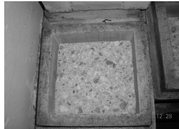
Fig. 5 – Cub spart – 100 mm beton – seria S16 / Broken cube – 100 mm of concrete – series S16
