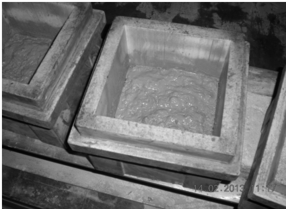
Fig. 4 – Cub spart – 50 mm beton – seria S15 / Broken cube – 50 mm of concrete – series S15.
