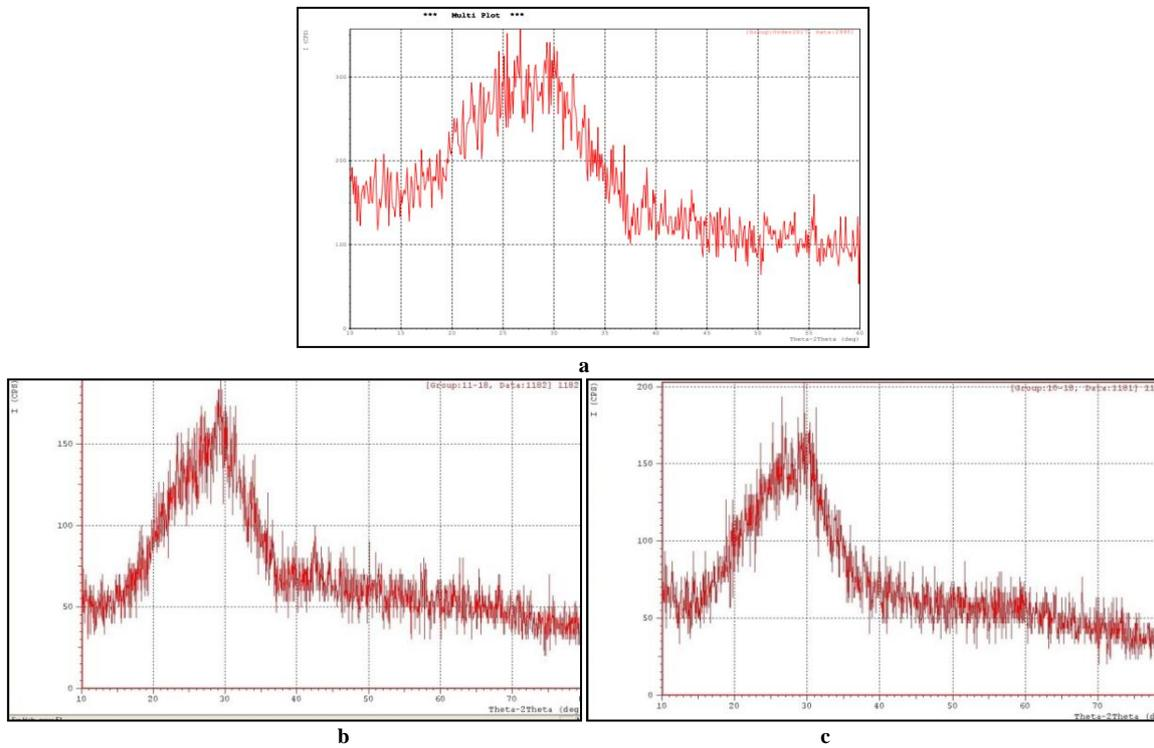
Fig. 5 - XRD patterns of a: MGP, b: MGP-K5 pastes, c: MGP-S pastes (cured 1 day at 60°C and up to 7 days at 20°C).
