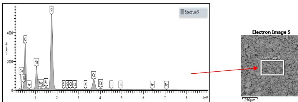
Fig.9 - SEM micrograph and EDS for MGP-S paste cured 24 h at 60°C and up to 7 days at 20°C.
