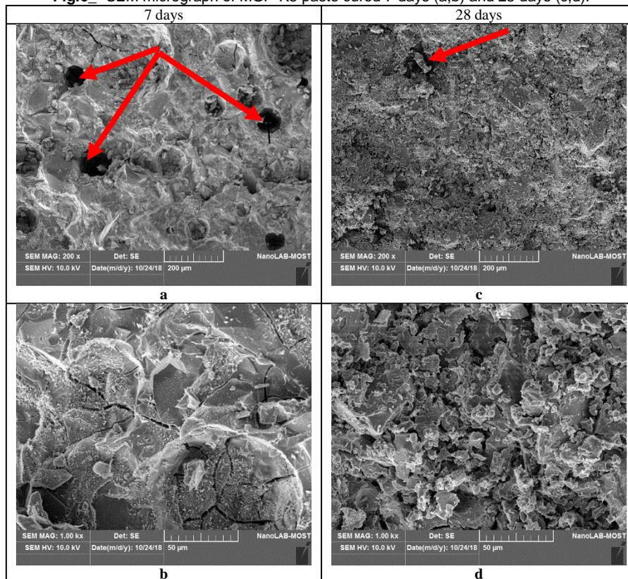
Fig.7\_ SEM micrograph of MGP-S paste cured 7 days (a,b) and 28 days (c,d).
