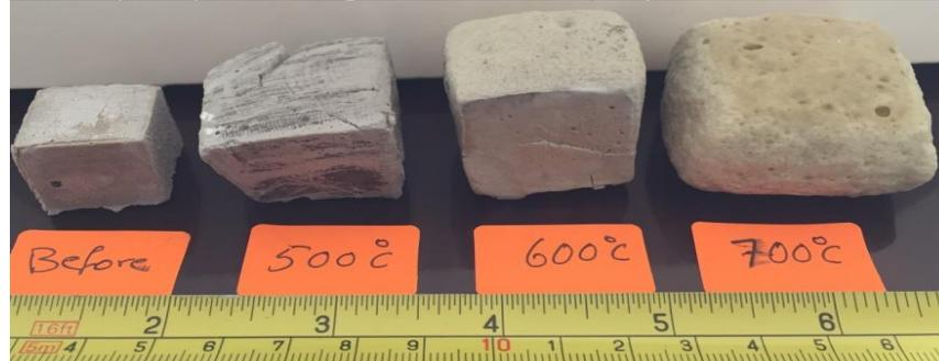
Fig.2 - MGP-S paste specimen's images before and after thermally treated at 500,600 and 700°C/1h
