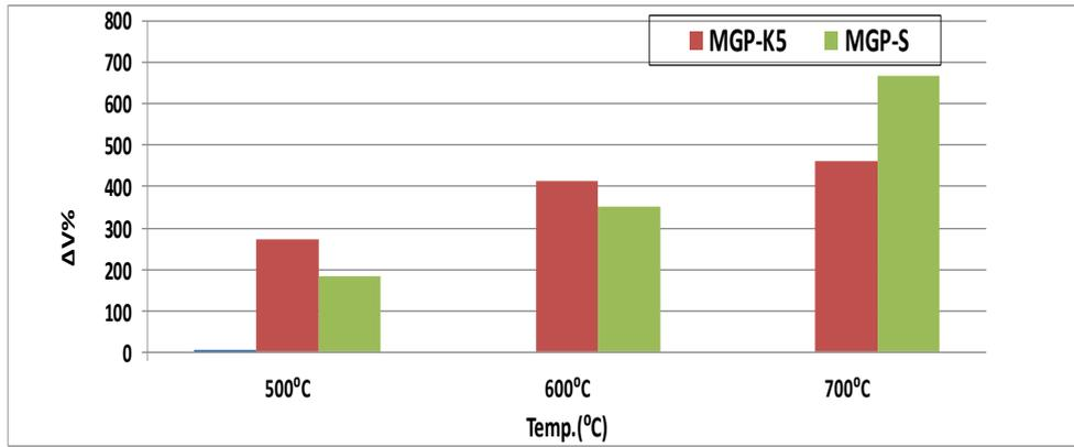
Fig.3 -Volume changes of MGP-K5 and MGP-S paste specimen's after thermally treated at 500,600and700°C/1 h.
