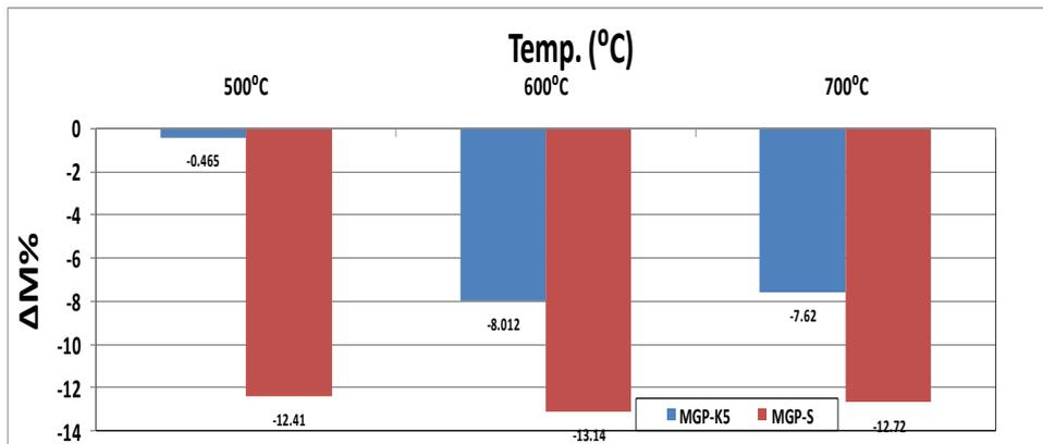
Fig.4 - Mass change of MGP-K5 and MGP-S paste specimen'safter thermally treated at 500,600and700°C/1 h.
