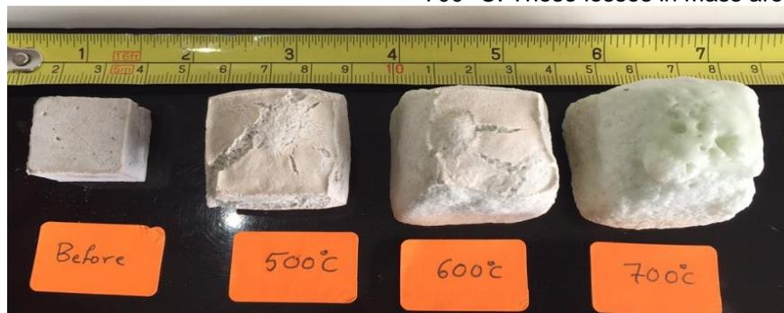
Fig.1 -MGP-K5 paste specimen's images before and after thermally treated at 500,600 and 700°C/1h.
