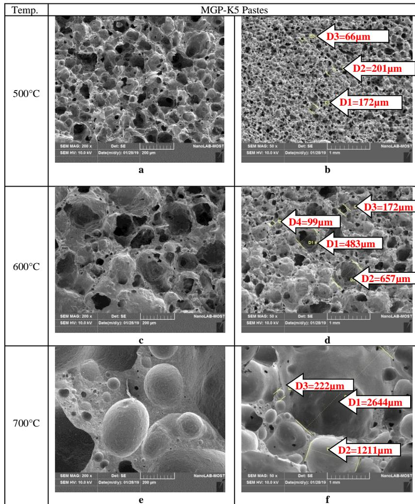
Fig.10 -SEM images of MGP-K5 paste specimens after thermally treated at temperatures 500,600 and 700°C (on fracture surface).
