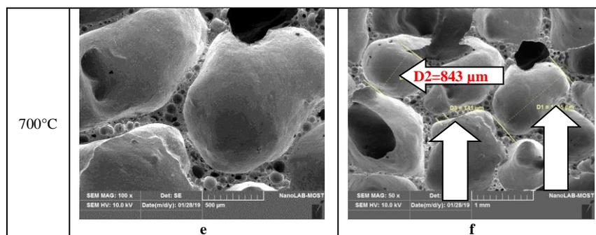
Fig.11 -SEM images of MGP-S paste specimens after thermally treated at temperatures 500, 600 and 700°C (on fracture surface).
