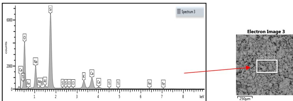
Fig.8 - SEM micrograph and EDS for MGP-K5 paste cured 24 h at 60°C and up to 7 days at 20°C.
