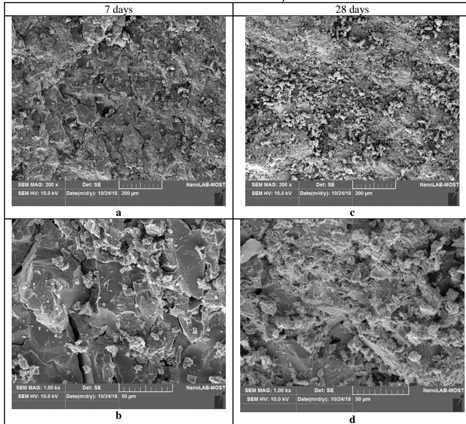
Fig.6\_ SEM micrograph of MGP-K5 paste cured 7 days (a,b) and 28 days (c,d).
