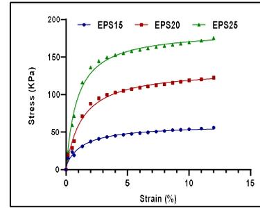
Fig.6c - Stress-strain curves for 150mm<sup>3</sup>
