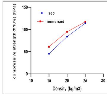
Fig.8 - Influence density on the compressive strength  $\sigma_{10\%}$
