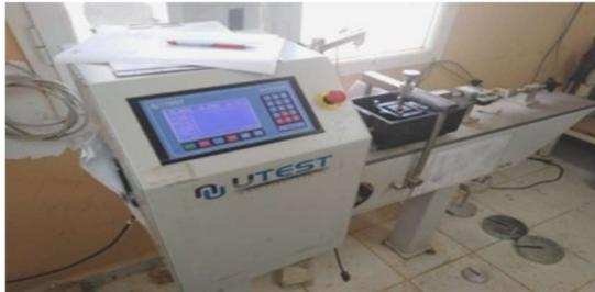
Fig.5 - Automatic shearing machine UTS-2060
