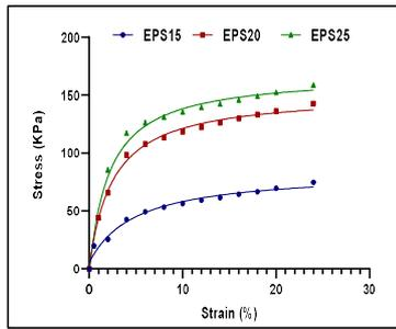
Fig.6a - Stress-strain curves for 50mm<sup>3</sup>
