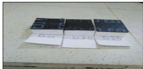
Fig.3 - Reinforced polystyrene samples
