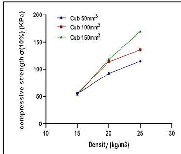
Fig. 7 - Variation compressive strength  $\sigma_{10\%}$  with density
