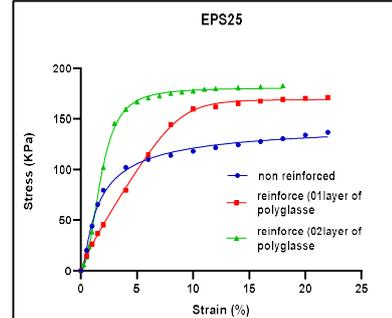
Fig.9 - Stress-strain behavior of EPS reinforced by polyglass
