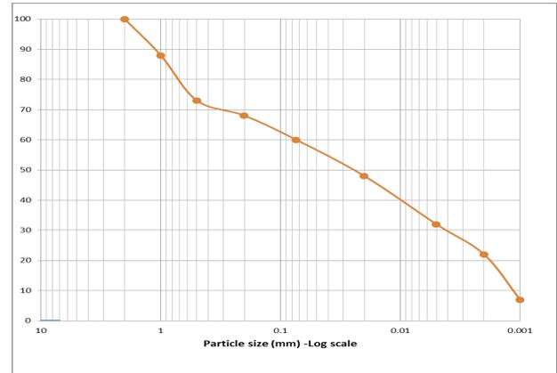
Fig. 4 – Grain-size distribution curve of the silty-sandy brown clay / Curba granulometrică a argilei brune nisiposo-pufoase.
