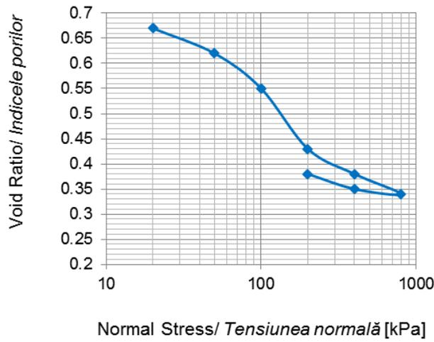
Fig. 10a - Consolidation curve of clay without bituminous oil shale ash/ Curba de consolidare a argilei brune.
