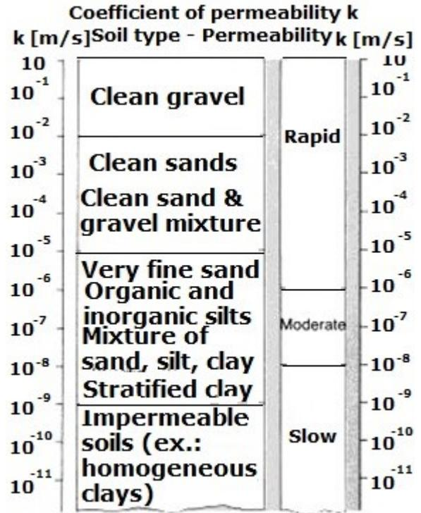
Fig.8 - Classification of the coefficient of permeability/ Clasificarea coeficientului de permeabilitate [34].
