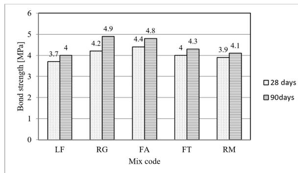
Fig. 6 - Comparison of bond strength by Pull-off test results at the age of 28 and 90 days.
