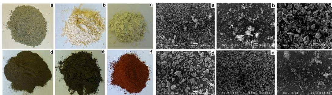
Fig. 1 - Photo (left) and SEM (right) display of used cement and mineral powder admixtures: a) cement, b) limestone filler, c) recycled cathode ray tube glass, d) fly ash, e) flotation tailings, f) red mud
