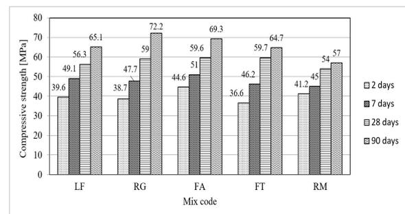
Fig. 3 - Comparison of compressive strength results at the age of 2, 7, 28 and 90 days.
