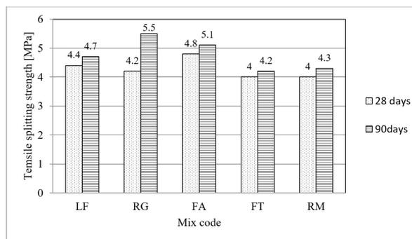
Fig. 5 - Comparison of tensile splitting strength results at the age of 28 and 90 days.
