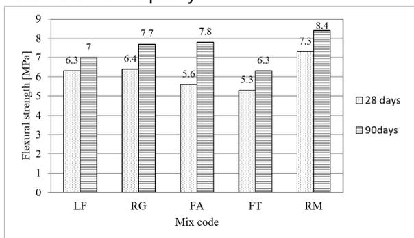
Fig. 4 - Comparison of flexural strength results at the age of 28 and 90 days.
