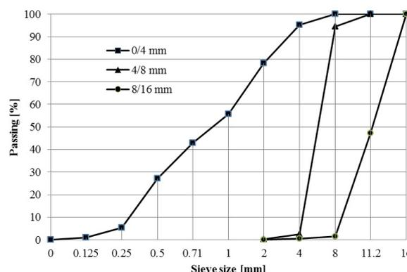
Fig. 2 - Particle size distribution of used aggregate
