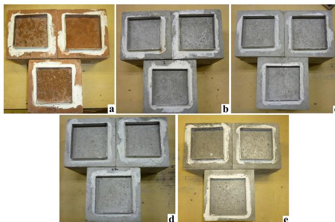
Fig. 8 - Appearance of the concrete surface after 28 freeze-thaw cycles with de-icing salt: a) RM, b) FT c) RG, d) LF and e) FA.
