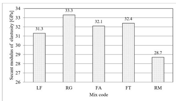
Fig. 7 - Comparison of secant modulus of elasticity at the age of 28 days.
