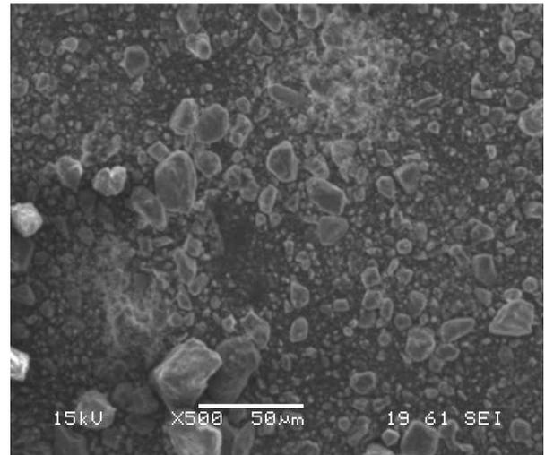
Fig.7. Scanning electron microscopic view of pozzolanic fillers after grinding
