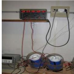
Fig. 2- Mounting system for the cell migration assay
