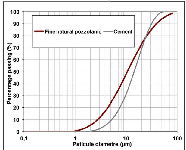
Fig. 5 - Granulometric analysis of cement and pozzolana
