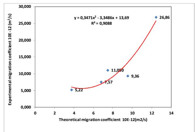
Fig. 16 - Theoretical and experimental chloride ion diffusion coefficients
