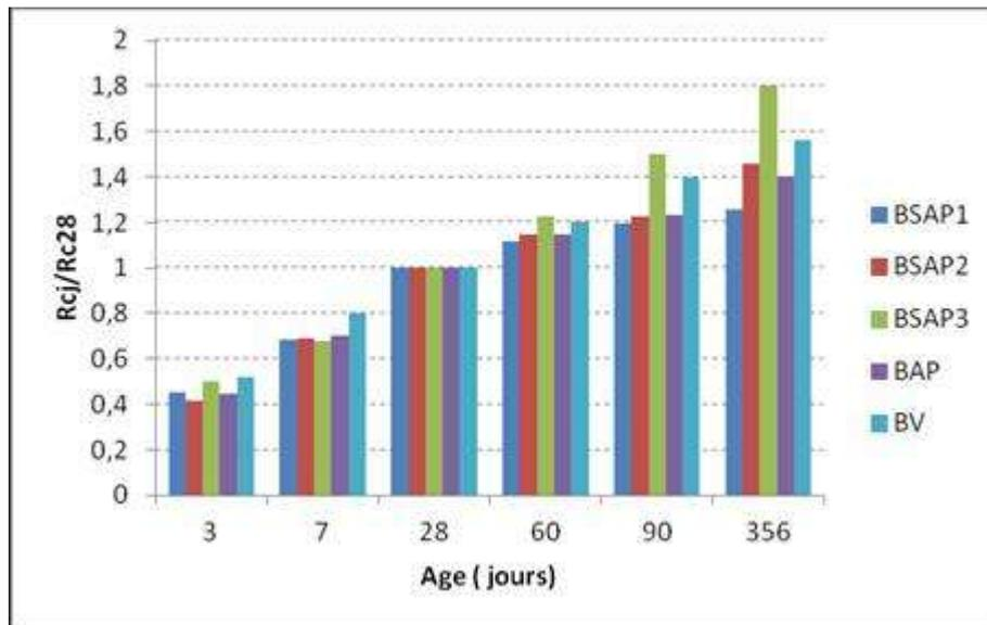
Fig.10. Evolution of the simple compressive strength of all concrete compositions under study
