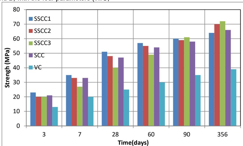
Fig. 9 - Evolution of the simple compressive strength of all concrete compositions under study
