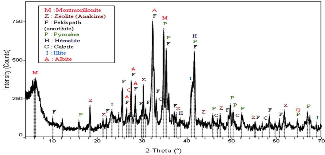
Fig. 6. X-ray diffraction spectrum of natural pozzolana (Beni-Saf)
