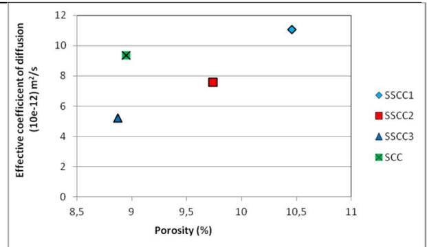
Fig. 14 - Diffusion coefficient as a function of porosity in our concretes
