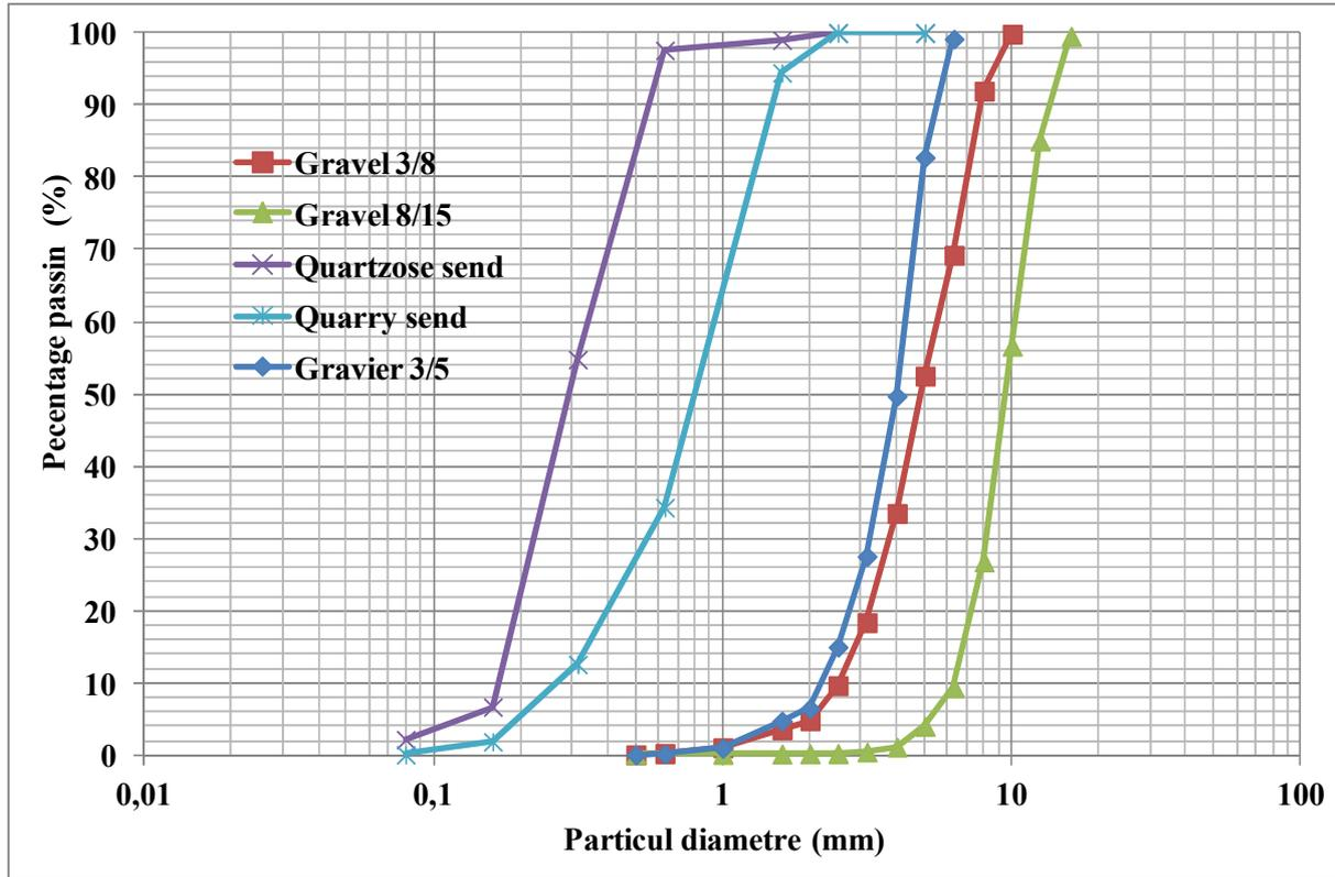
Fig.4 - Granulometric analysis of aggregates
