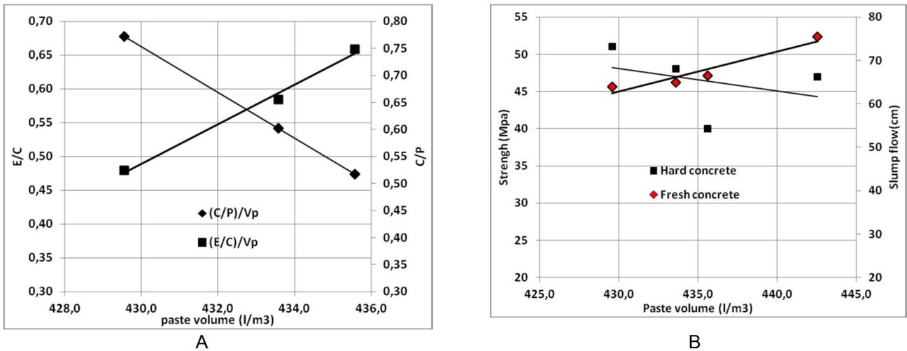
Fig. 8 - **A.** Influence of W/C and C/P ratios on paste volume, **B.** Influence of paste volume on fresh and hardened states of SCSC and SCC.
