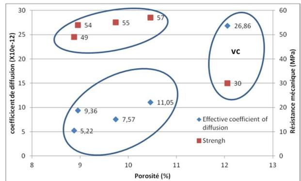
Fig. 15- Coefficient of chloride ion diffusion as a function of the compressive strength of the different concretes
