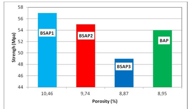
Fig 12 - The compressive strength at 28 days of the different types of concrete as a function of the open porosity.
