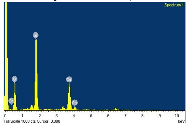
Fig. 12 - EDS of sample with 2% NS
