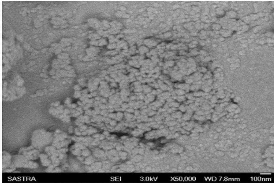
Fig. 1 - SEM image of nano SiO<sub>2</sub>.
