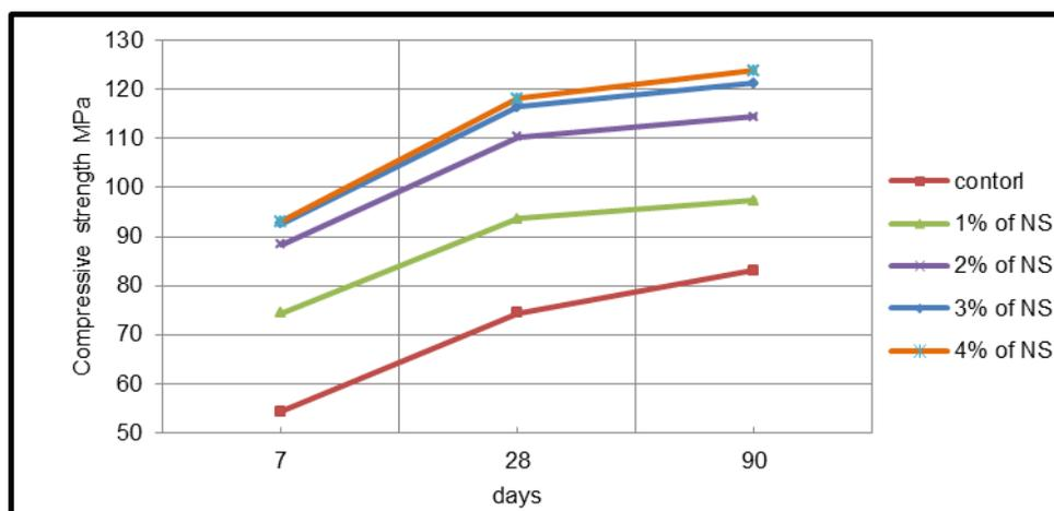
Fig. 5 - Effect of nano silica on compressive strength.
