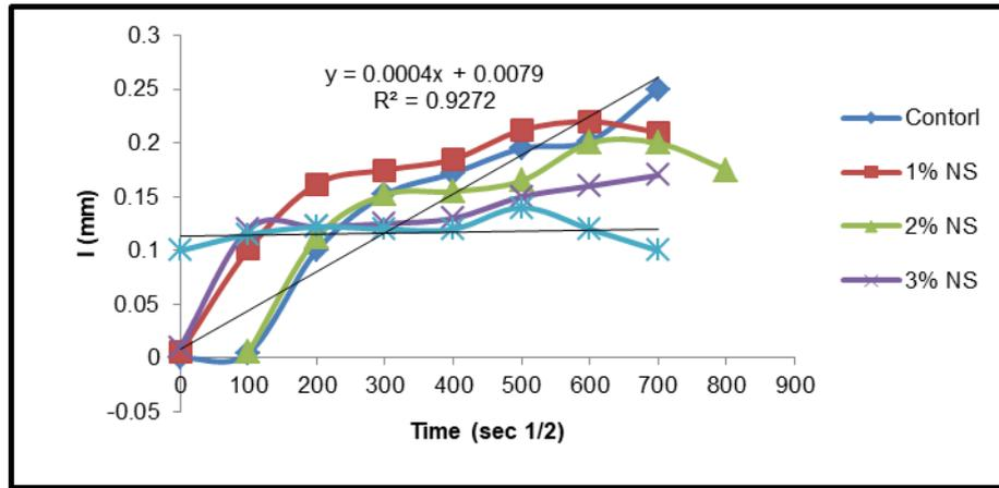
Fig. 7 - Effect of nano silica admixture sorptivity
