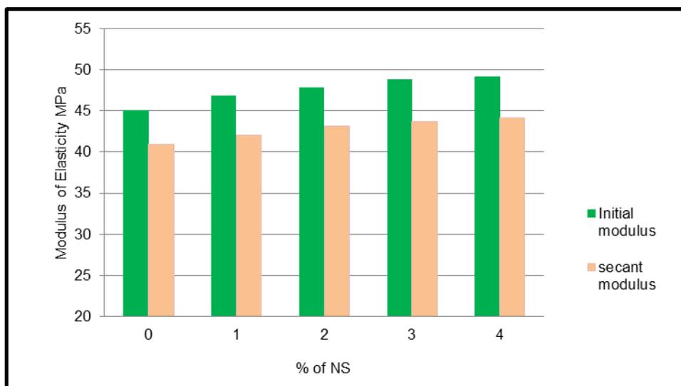
Fig. 6 - Effect of nano silica admixture on modulus of elasticity.
