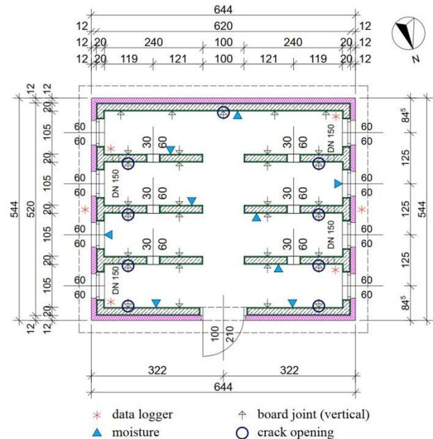
Fig. 5 - Ground plan of the building (dimensions in cm) with north arrow and position of the monitoring points.
