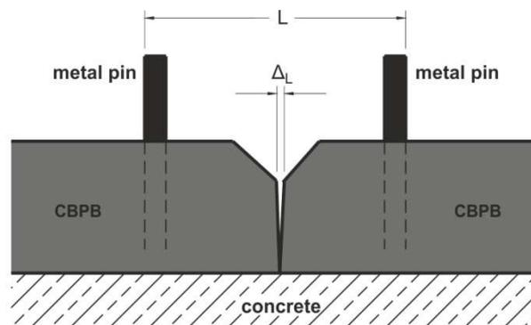
Fig. 7 - Setup for the measuring of the crack opening in the board joints.
