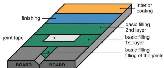
Fig. 1 - Schematic Illustration of the layers of the tested complete coating systems.
