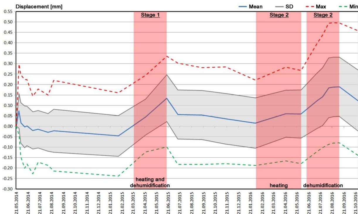
Fig. 10 - Crack opening in the board joints during the monitoring of the building.
