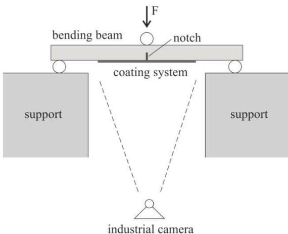
Fig. 2 - Schematic illustration of the setup of the used test method for strain and CBA measurements of coating systems acc. to patent [16].
