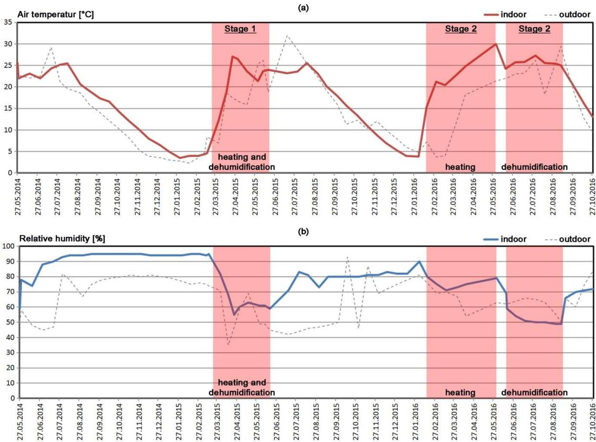
Fig. 8 - Air temperature (a) and relative humidity (b) during the monitoring of the building.
