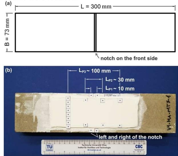
Fig. 3 - Shape and dimensions of the bending beams (a) and a bending beam ready for testing with point pattern (b) acc. to patent [16].
