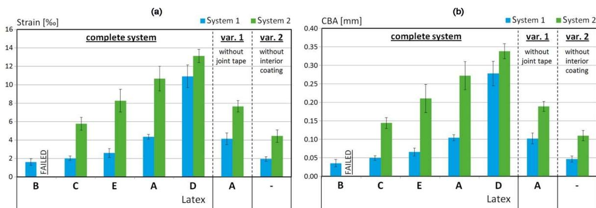
Fig. 4 - Strain (a) and crack-bridging ability (CBA) (b) of the tested coating systems.
