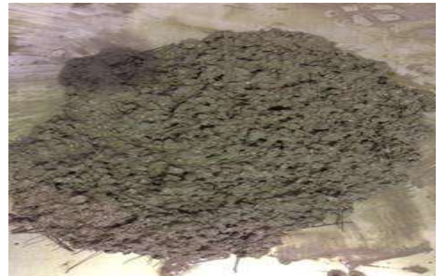
Fig. 1 - Typical mix with 0.50 % steel fiber addition.
