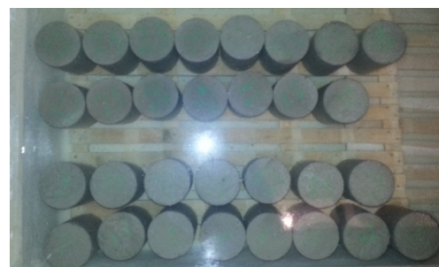
Fig. 2- Curing of concrete cylinders / Maturarea epruvetelor cilindrice.
