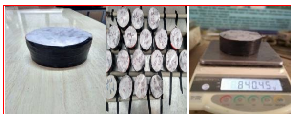
Fig. 3 - Sorptivity Test performed after 28 and 90 days.
