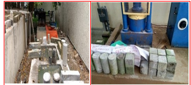
Fig. 2 - Water Absorption test on concrete cubes
