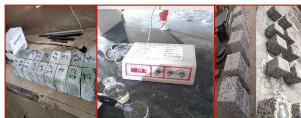
Fig. 4 - Acid Attack test performed after 28 and 90 days.
