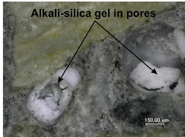
Fig. 7- Pores completely filled by alkali-silica gel near the reactive quartz, x50.
