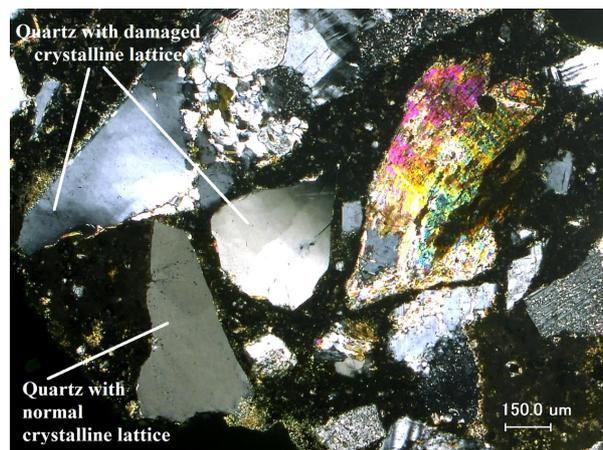
Fig. 2 – Quartz with damaged crystalline lattice, x50
