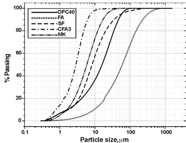
Fig. 1 - Particle size distribution of the artificial pozzolans.
