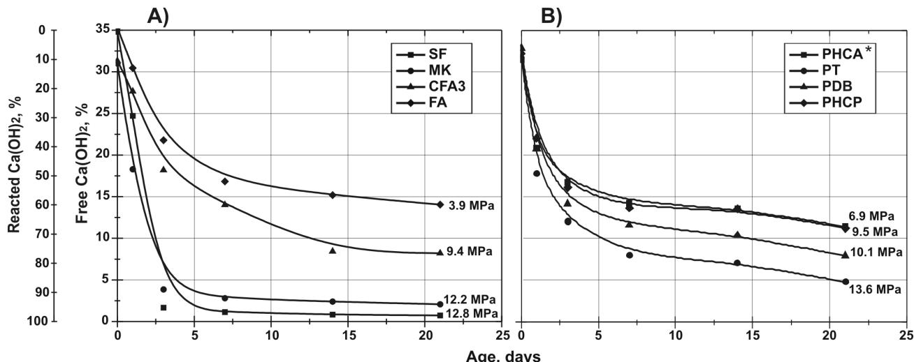
Fig. 3 -  $\text{Ca}(\text{OH})_2$  consumption obtained by the Modified Franke Test Method for 1, 3, 7, 14 and 21 days. (A) Results from artificial pozzolanas; (B) Results from natural pozzolanas adapted from [5]. Strength data: Mortars at 7 days of curing. \*Abbr: no specific meaning
