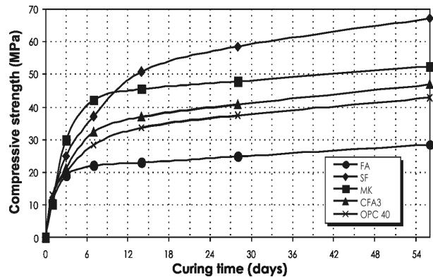
Fig. 4 - Strength of partially replaced Portland cement mortars (20% pozzolan) cured at 23±2°C.
