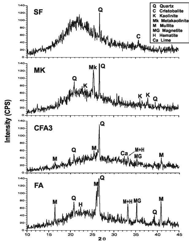
Fig. 2 - XRD patterns of the artificial pozzolans.
