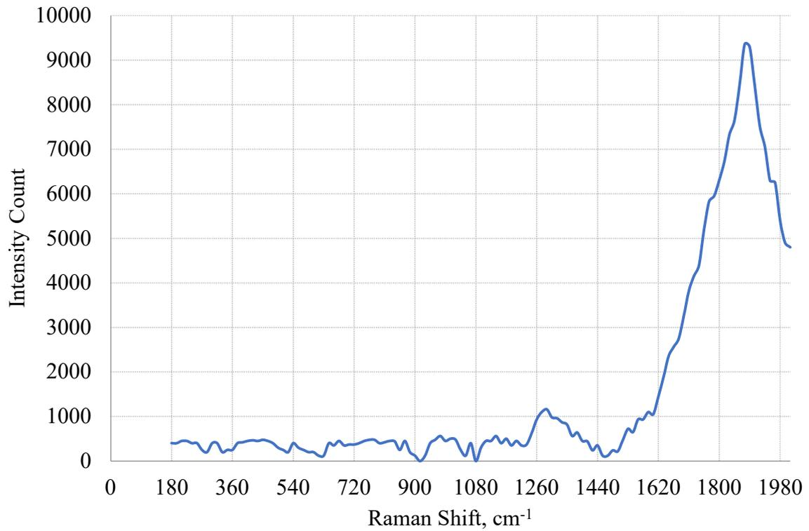
Fig. 7 - RAMAN spectrum of the carbon film (S=2mm, W=5,23 J, f=50Hz) / . Spectrul RAMAN al filmului de carbon (S=2mm, W=5,23 J, f=50Hz)
