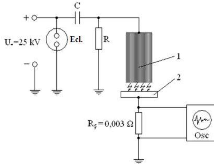
Fig. 1 - Schematic presentation of the experimental stand / Schema standului experimental
