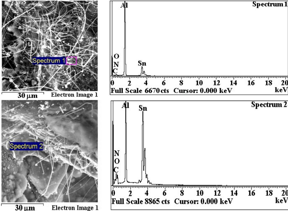
Fig. 3 - Morphology and EDX spectra of the electrode-anode and workpiece-cathode surfaces after processing
