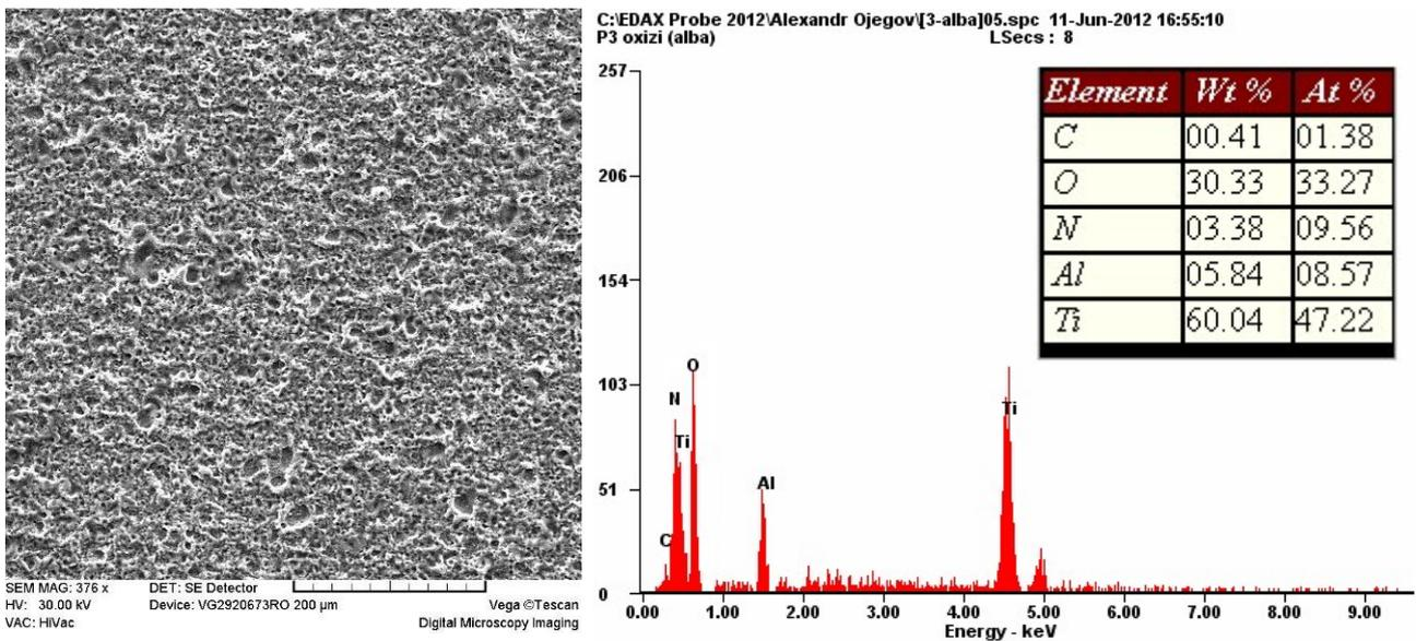
Fig. 12 - Morphology (SEM) and composition (EDX) of surfaces of samples executed by titanium alloy BT8 and processed by PEDM
