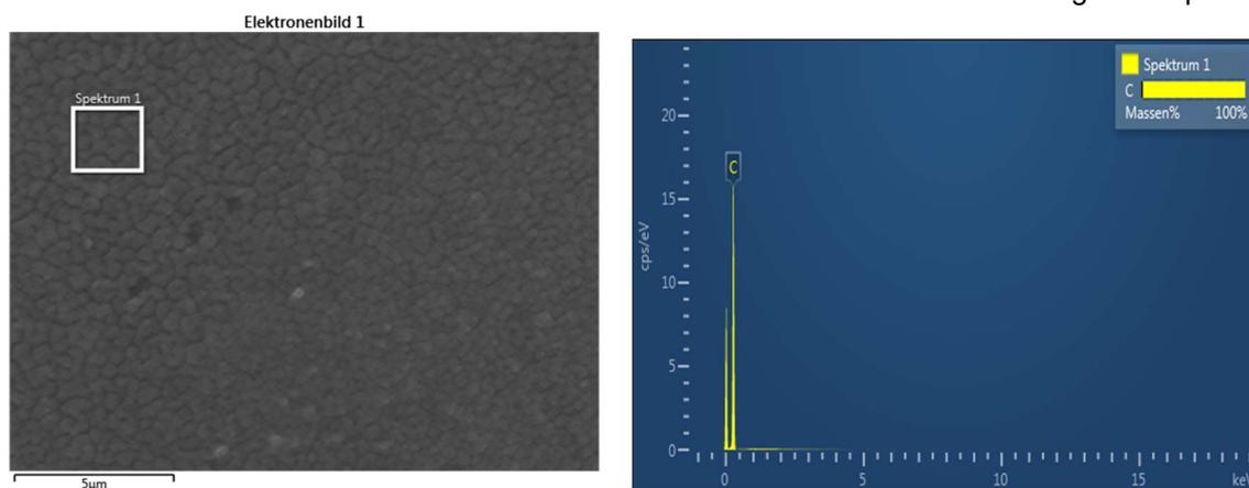
Fig.4 - Surface morphology of tool electrode (a) and chemical composition of tool material (b)
