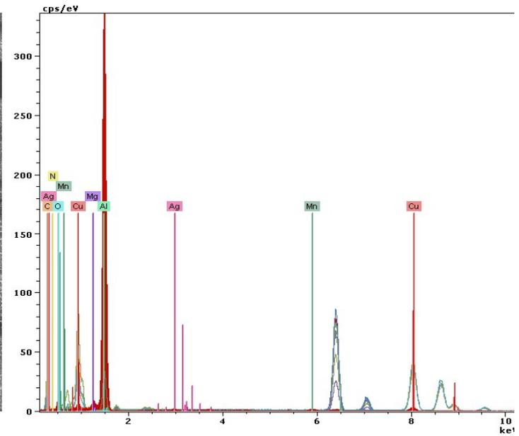
Fig. 13 - Morphology (SEM) and composition (EDX) of sample surfaces executed by aluminum alloy D16 and processed by PEDM
