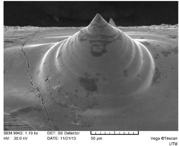
Fig.2 - Conical meniscus view extracted from anode executed from W+10%Re (energy released into the gap W = 3,04J, capacitor battery capacity of generator C = 200µF, gap size S = 0,3 mm, diameter of machined surface area d = 0,25 mm, number of electrical discharges applied to surface portion n = 1) / *Asperitate conică extrasă din suprafața anodului executat din aliajul W+10%Re*
