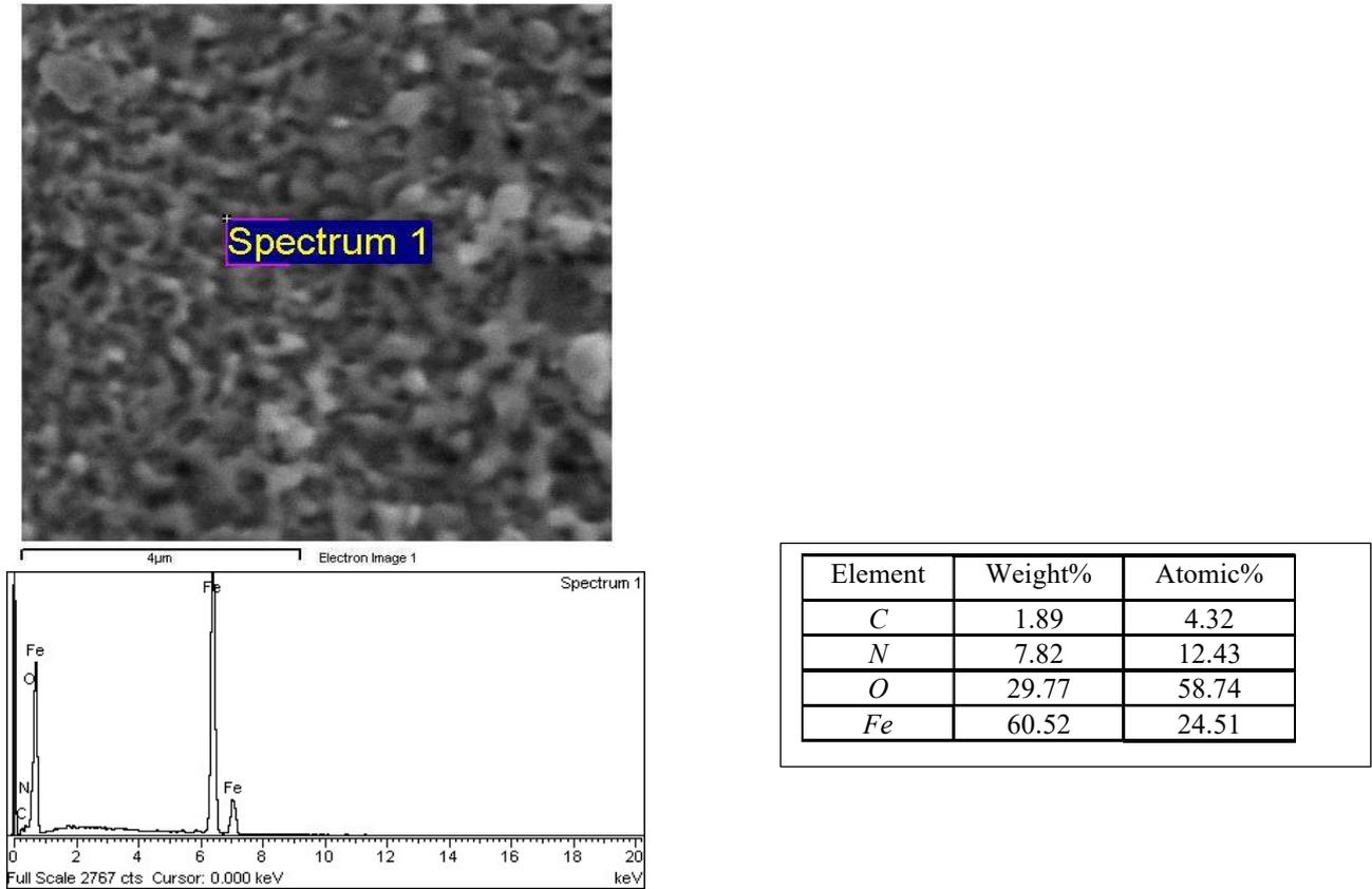
Fig. 11 - Morphology (SEM) and composition (EDX) of surfaces of samples executed by Steel 45 and processed by PEDM.
