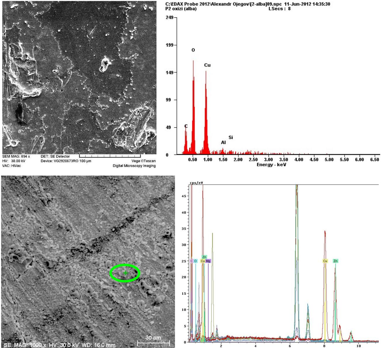
Fig. 14 - Morphology (SEM) and composition (EDX) of surfaces of samples executed by copper alloy and processed by PEDM : 1 – pure copper of brand M0; 2 – bronze based on aluminum brand BrA5; 3 – brass brand L63 / . *Morfologia (SEM) si compozitia (EDX) suprafetelor pieselor executate din aliaje ale cuprului si prelucrate cu aplicarea PDEI*
