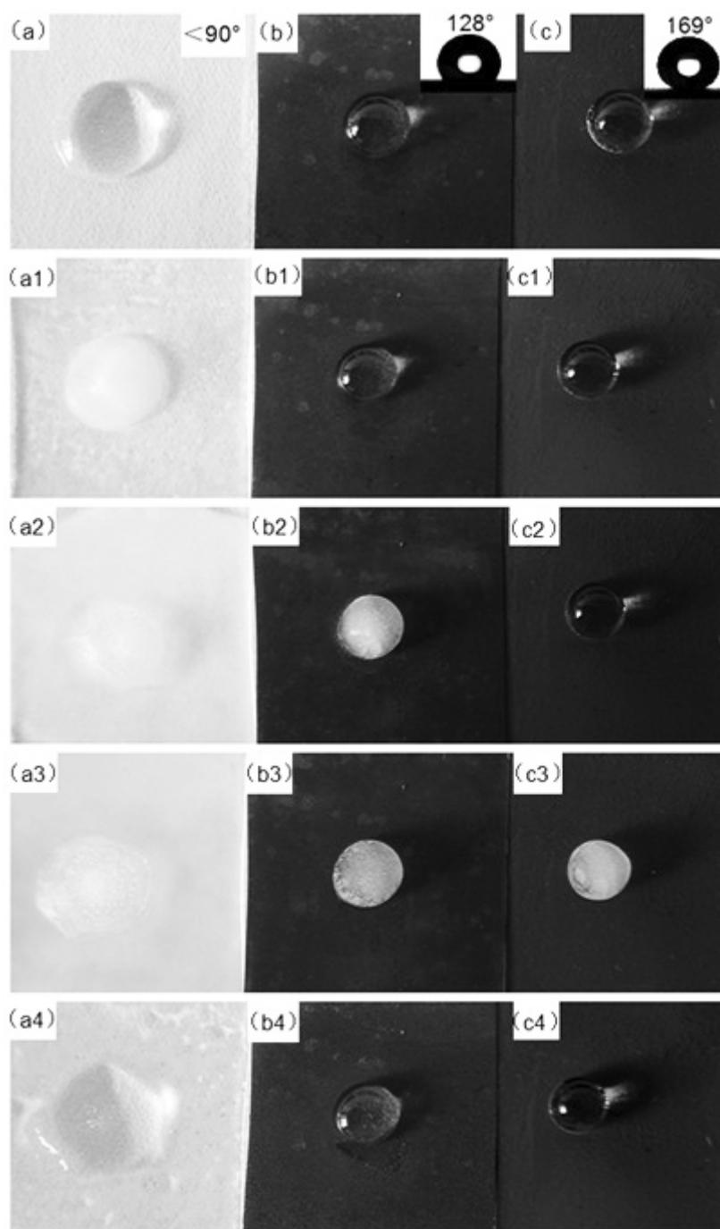
Fig. 4 - Select photographs of freeze process of water droplets on the three different surfaces at  $-5^\circ\text{C}$ . (a) common smooth surface, (b) hydrophobic  $\text{Co}_3\text{O}_4$  films surface, (c) superhydrophobic  $\text{Co}_3\text{O}_4$  films surface
