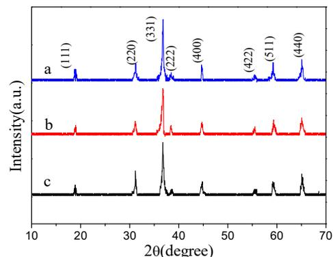
Fig. 1 - XRD patterns of the Co<sub>3</sub>O<sub>4</sub> film samples: (a) sample with adding CTAB for 60 min; (b) sample with adding CTAB for 90 min; (c) sample without adding CTAB for 90 min.
