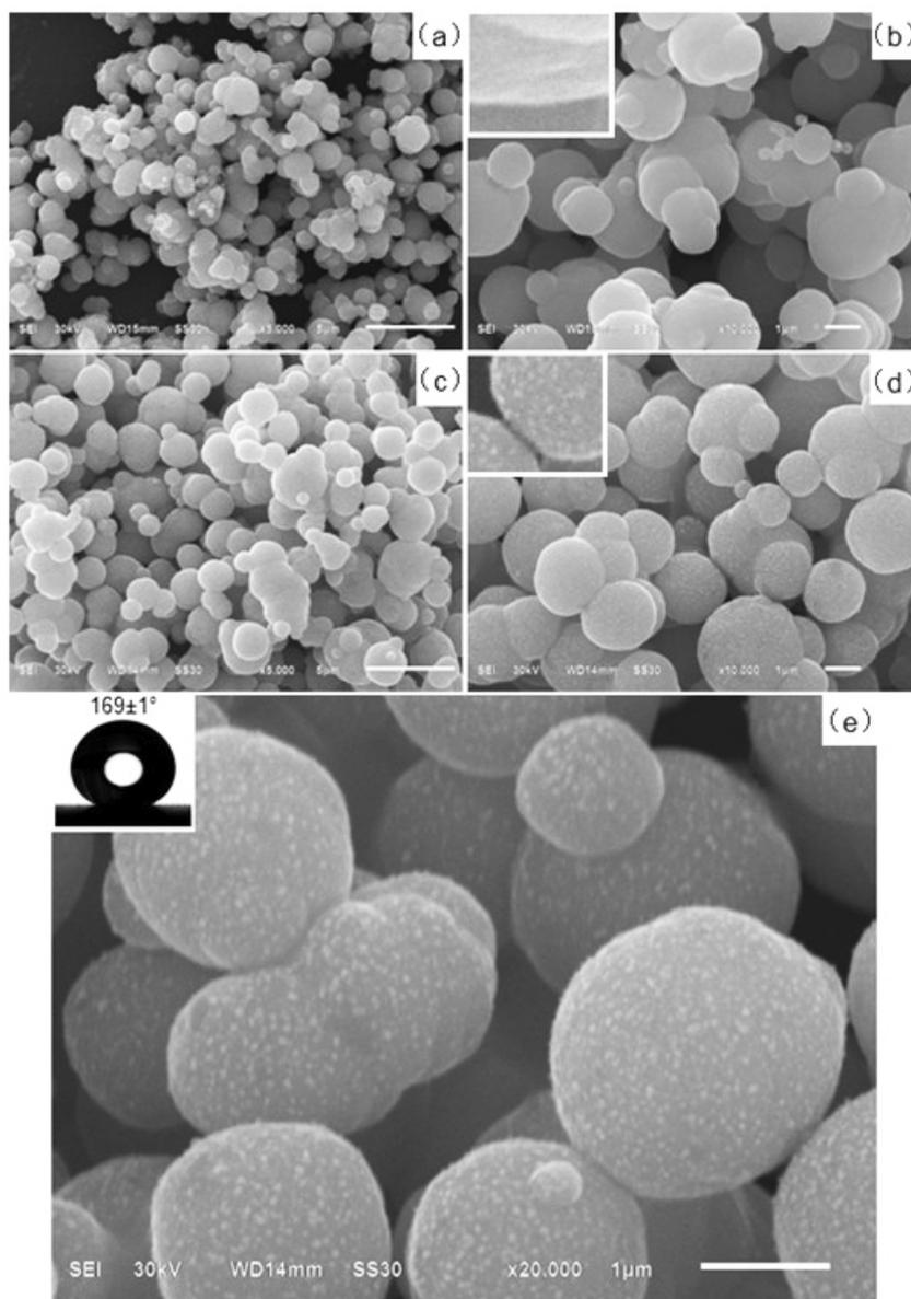
Fig. 2 - SEM images of the  $\text{Co}_3\text{O}_4$  film samples: (a),(b) sample for 60 min at low magnification and at high magnification, respectively; (c),(d) sample for 90 min at low magnification and at high magnification, respectively; (e) modified sample for 90 min
