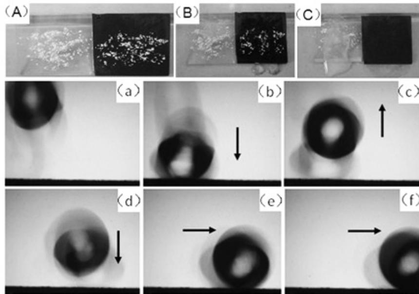
**Fig. 3** - Photographs (A, B and C) of self-cleaning process. Snapshots (a-f) of the dynamic behavior of a water droplet on the superhydrophobic  $\text{Co}_3\text{O}_4$  films with slightly tilted.
