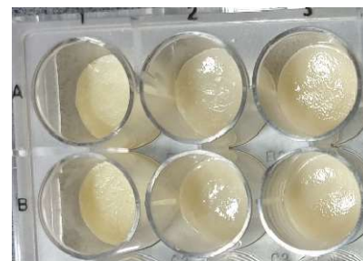
Fig.1- Initial pills from GRADIA® DIRECT Posterior Pastilele inițiale din GRADIA® DIRECT Posterior and a height of 2 mm was calculated and the value of 367.56 mm 3 was obtained. Considering that the manufacturer gives us the density of the Gradia® Direct Posterior composite as 1.9 g/cm 3 , by calculation we obtained the ideal weight of a correctly molded tablet as well as homogeneity and thickness as 0.698 g [15]. By weighing and measuring the thickness we ensured that each tablet was cast evenly.
