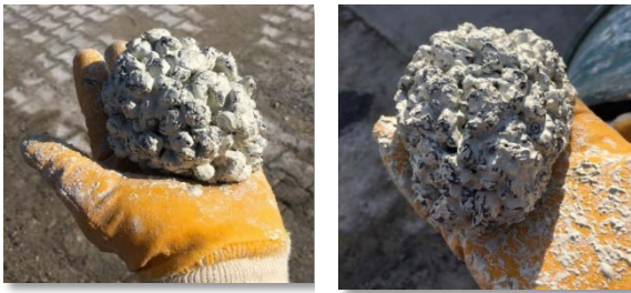
Fig 5. As a result of the pervious concrete consistency test, the mixtures that stayed in snowball form
