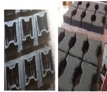
Fig.2 - Casting of specimen
