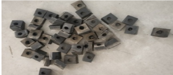
Fig.1 -10mm diameter hole on the surface of the reshaped tyre rubber
