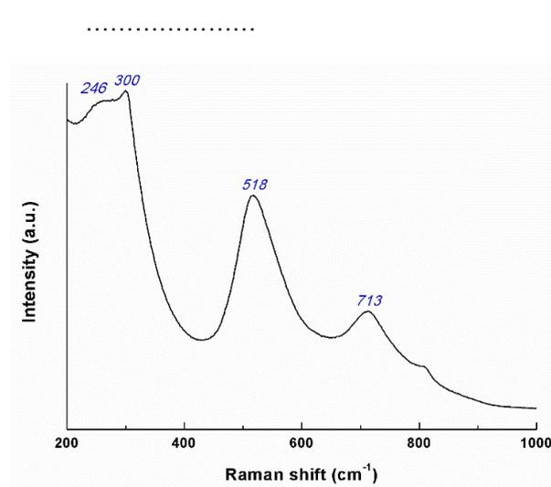
Fig. 2 - Raman spectrum of BT powder.
