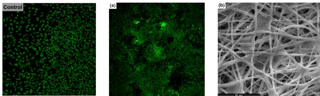
Fig. 5 - (a) Fluorescence microscopy and (b) SEM images recorded on PCL-HA-BT scaffold.
