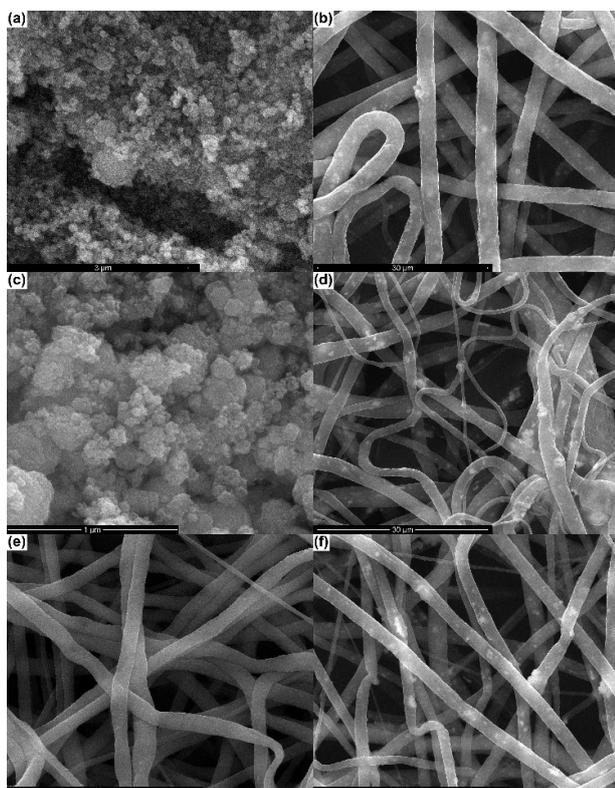
Fig. 3 - SEM images of: (a) HA powder, (b) PCL-HA scaffold, (c) BT powder, (d) PCL-BT scaffold, (e) PCL scaffold and (f) PCL-HA-BT scaffold.
