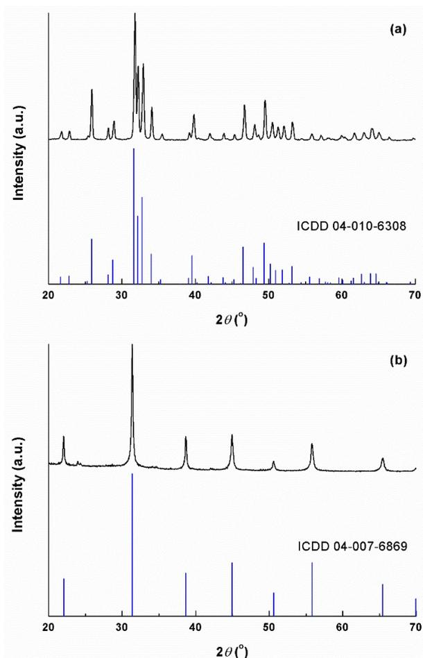
Fig. 1 - XRD patterns of: (a) HA powder and (b) BT powder, compared to the standard patterns from the database.
