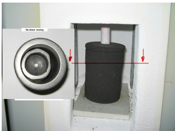
Fig. 4 – Ansamblu de grafit / Graphite assembly.
