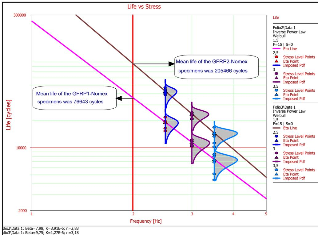
Fig. 12 – The graphical method for determining the mean number of cycles for the GFRP1-Nomex and GFRP2-Nomex specimens/
