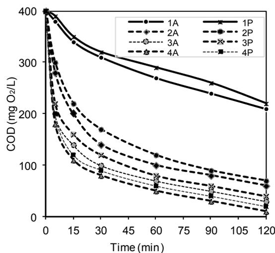
Fig. 3a - Photocatalytic activity of  $\text{Fe}_3\text{O}_4\text{-TiO}_2$  nanoparticles / *Activitatea fotocatalitică a nanoparticulelor  $\text{Fe}_3\text{O}_4\text{-TiO}_2$ .*
