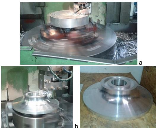
Fig. 4 - The machining process of the duralumin block / Prelucrarea blocului de duraluminu
