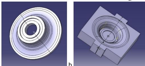
Fig. 3 - Mould components – 3D CAD model / Componentele matriței – model 3D CAD.
