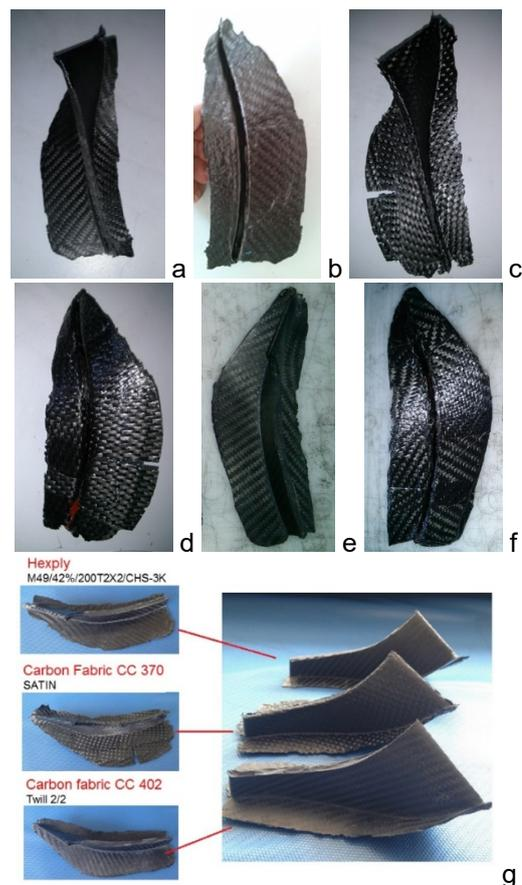
Fig. 17 - Rotor blades 1:1 scale - technological trials: a, b) HexPly M49 blade; c, d) CC370 blade; e, f) CC402 blade; g) all three rotor blades / Paletele de rotor scara 1:1 – teste tehnologice: a, b) Paleta din HexPly M49; c, d) Paleta din CC370; e, f) Paleta din CC402; g) Cele trei palete de rotor.
