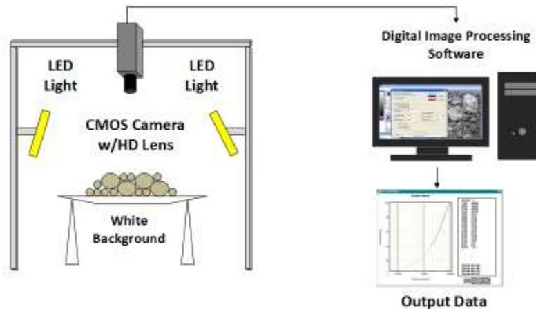
Fig. 1 - Schematic view of the lab set-up.
