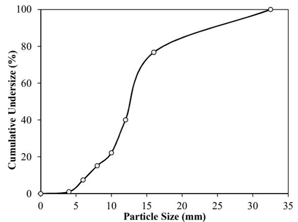
Fig. 7 - Result of PSD analysis using sieving method.
