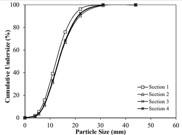
Fig. 8 - Result of PSD analysis using DIP method.
