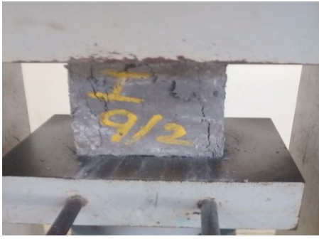
Fig. 12 - Failure of HFRC specimen.
