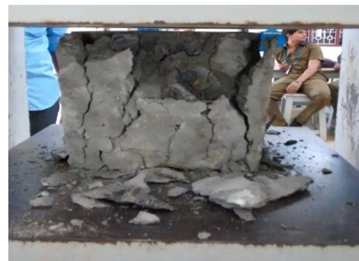
Fig. 11 - Failure of control specimen.
