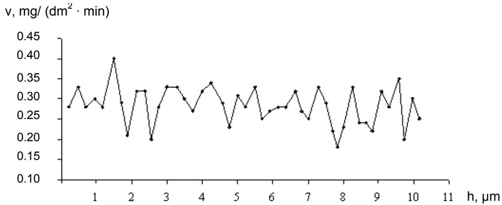
Fig.1- Rate of dissolution of flat glass. The samples were kept in HF solution in stationary position. Duration of one etching -20 minutes.
