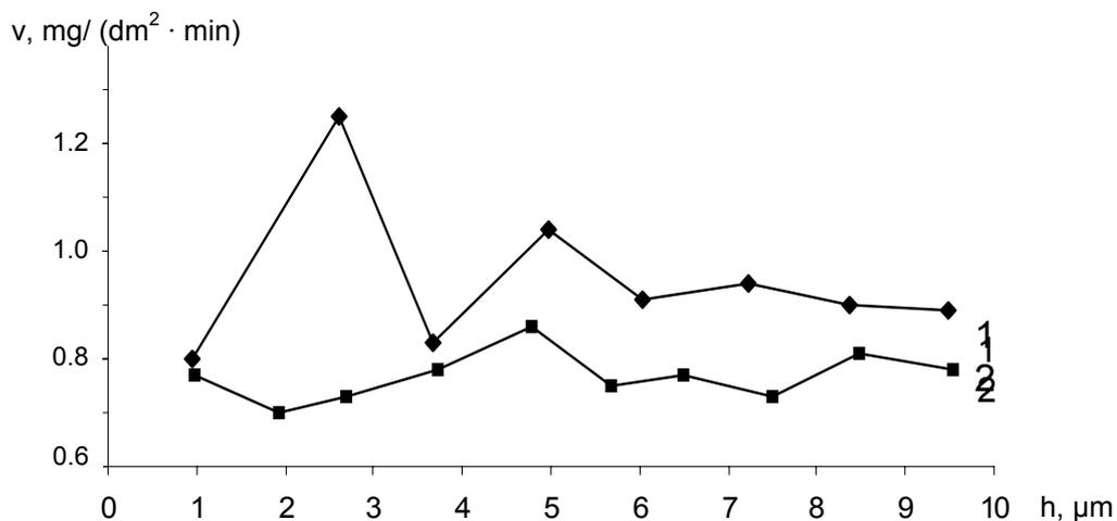
Fig.3 - Rate of dissolution of flat glass. The samples were rotated in the HF solution. Duration of one etching -10 minutes.
