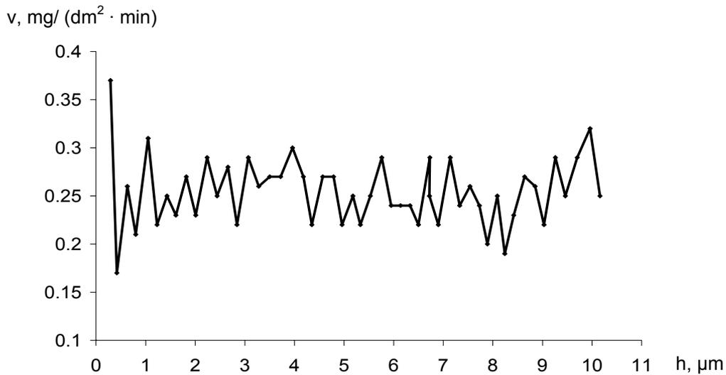
Fig.2 - Rate of dissolution of container colorless glass. The samples were kept in HF solution in stationary position. Duration of one etching -20 minutes.
