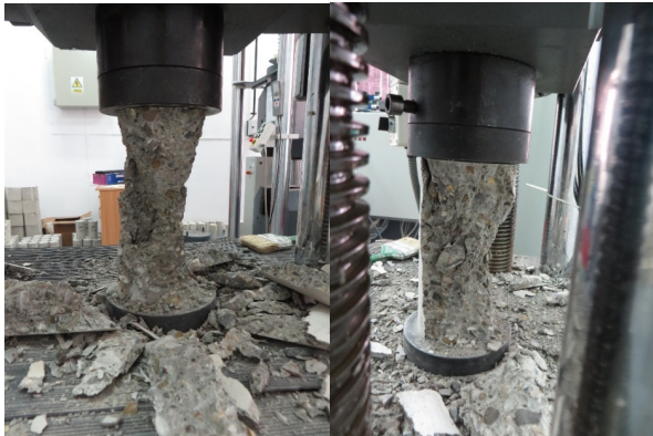
Fig. 4 – Failure of the cylindrical concrete specimens loaded in compression/ Cedarea probelor cilindrice din beton la compresiune.
