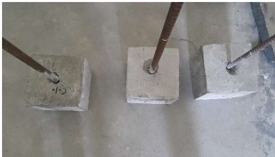
Fig. 4 - Failure of specimens in shear due to pull out of bars.
