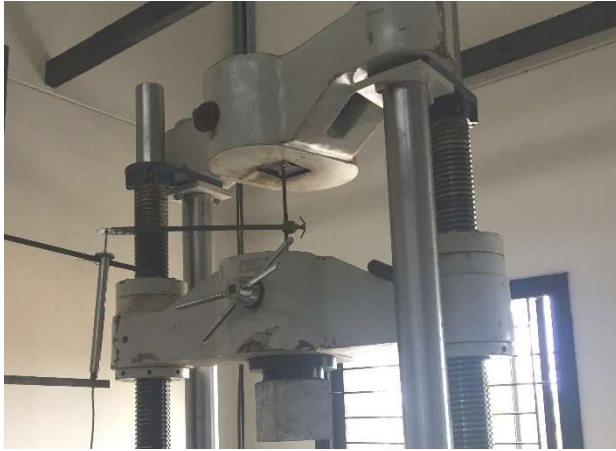
Fig. 3 - Testing of pull out specimens.
