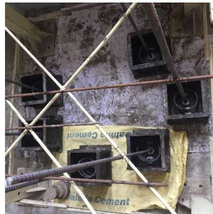
Fig. 2 - Casting arrangement of pull out specimens for 135 mm concrete cover
