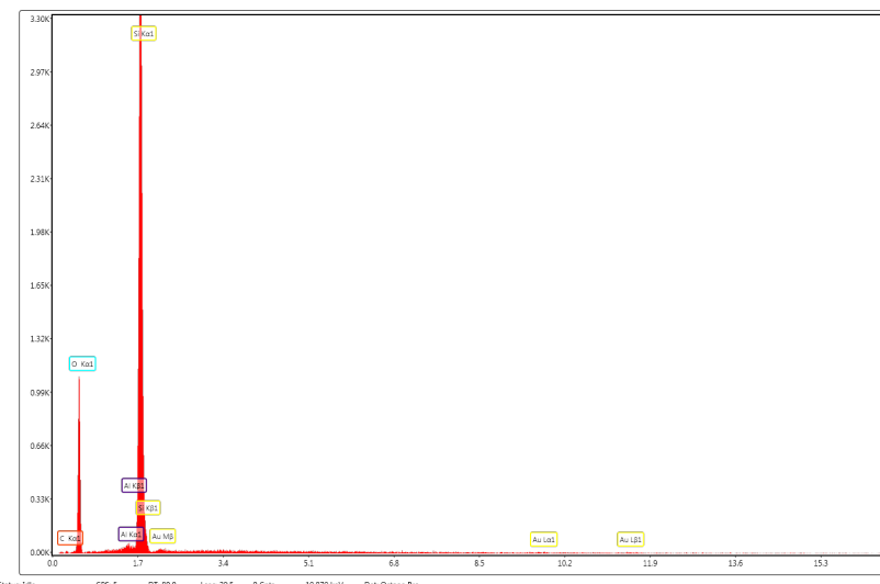
Fig. 5(b) - EDAX spectrum of post-calcined HZSM-5 catalyst / Spectrul EDAX a catalizatorului HZSM-5 postcalcinat.
