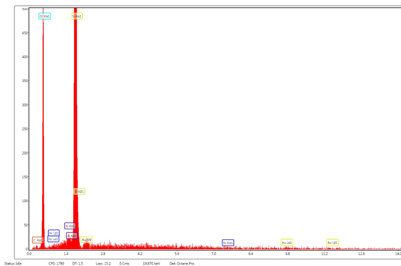
Fig. 6(a) - EDAX spectrum of pre-calcined HZSM-5 catalyst / Spectrul EDAX a catalizatorului Ni-ZSM-5 precalcinat.
