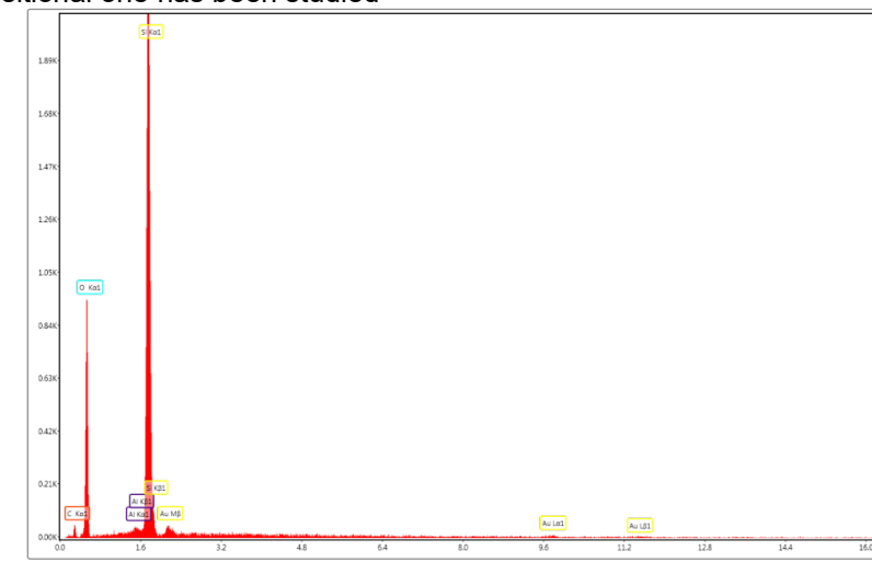
Fig. 5(a)- EDAX spectrum of pre-calcined HZSM-5 catalyst / Spectrul EDAX a catalizatorului HZSM-5 precalcinat.
