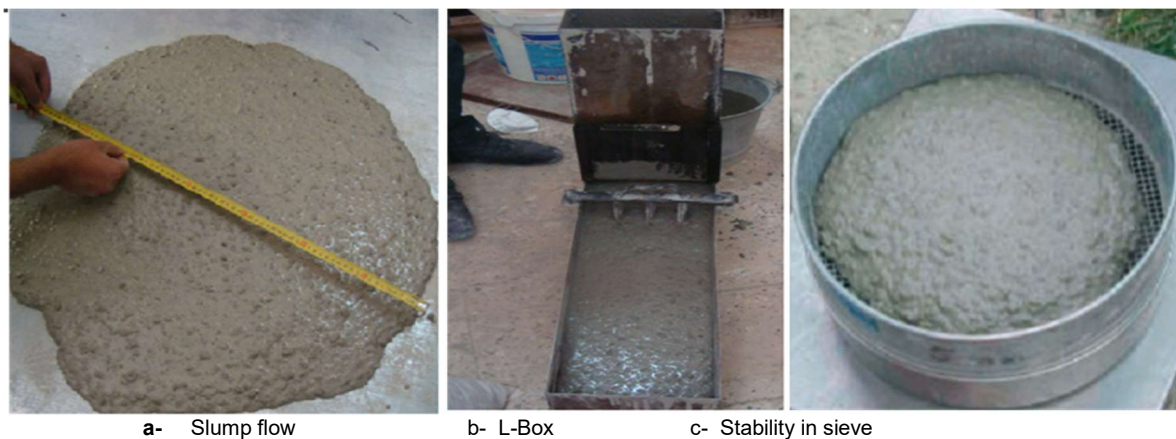
Fig. 3 - Qualification test of self-compactability concrete
