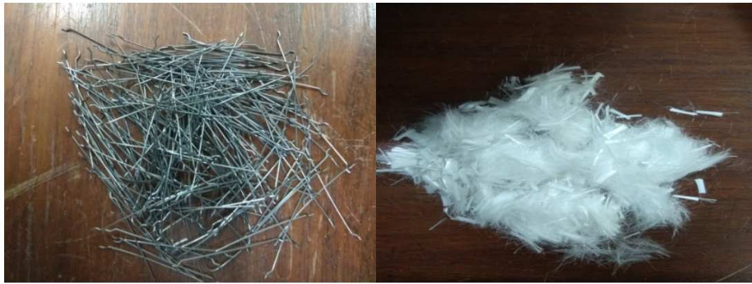
Fig.1 - Shape and dimensions of (a) Steel fibre (b) Polypropylene fibre.
