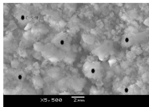
Fig.18 - 3-1-3 Interfacial transition zone SEM morphology (3d, W/B=0.34).
