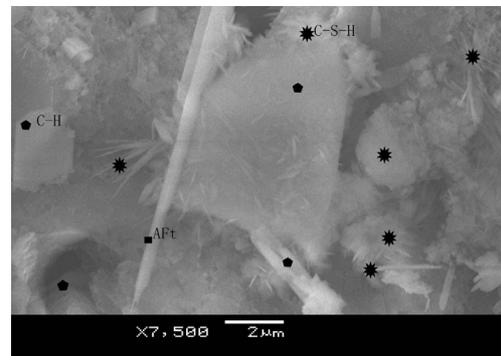
Fig. 17 - 3-1-1 Interfacial transition zone SEM morphology (3d, W/B=0.34).
