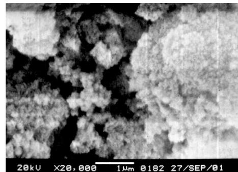
Fig.1 - Microscopic morphology of nano-SiO<sub>2</sub>.
