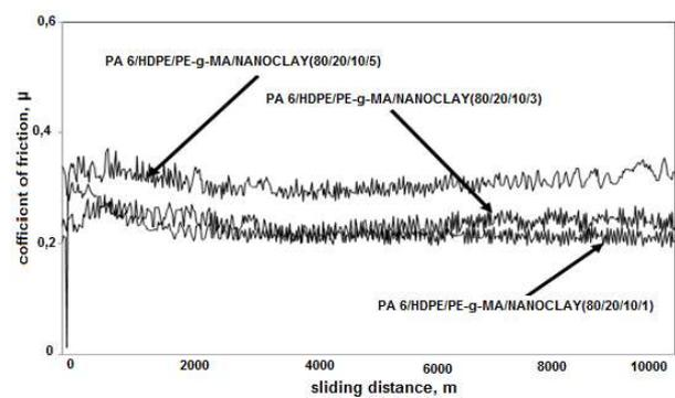
Fig. 10 - Coefficient of friction-sliding distance graph of PA 6/HDPE/PE-g-MA/Nanoclay (80/20/10/1), PA 6/HDPE/PE-g-MA/Nanoclay (80/20/10/3), PA 6/HDPE/PE-g-MA/Nanoclay (80/20/10/5) materials (load: 80 N, sliding speed: 1 m/s).
