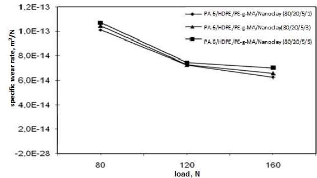
Fig. 6 - Variation of wear rate at applied load PA 6/HDPE/PE-g-MA/Nanoclay (80/20/5/1), PA 6/HDPE/PE-g-MA/Nanoclay (80/20/5/3), PA 6/HDPE/PE-g-MA/Nanoclay (80/20/5/5) nano composites tested against stainless steel (velocity: 1 m/s)
