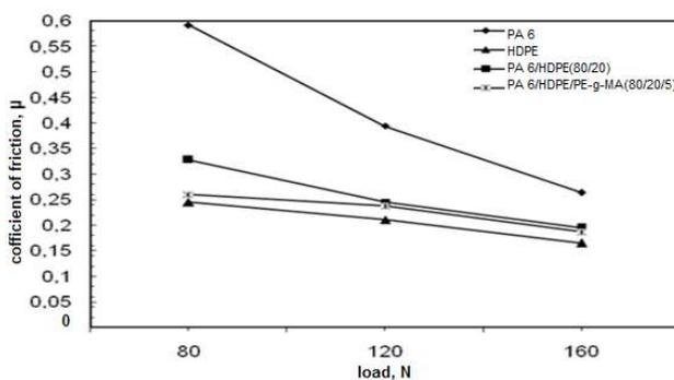
Fig. 2 - Variation of coefficient of friction with applied load for pure PA 6, pure HDPE, PA 6/HDPE (80/20), PA 6/HDPE/C (80/20/5) composites tested against stainless steel (velocity:1 m/s).
