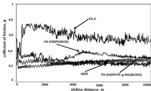
Fig. 8 - Coefficient of friction-sliding distance graph of PA 6, HDPE, PA 6/HDPE (80/20), PA 6/HDPE/ PE-g-MA (80/20/5) materials (load: 80 N, sliding speed: 1 m/s)
