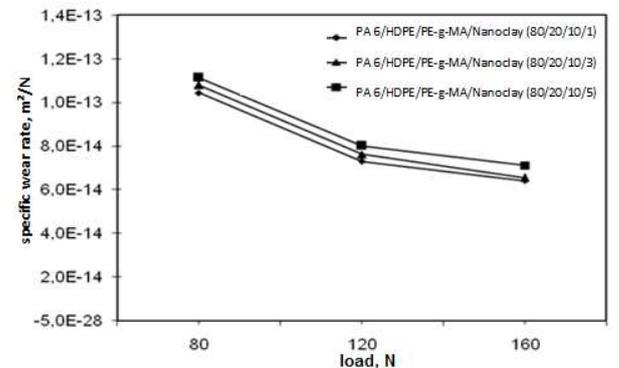
Fig. 7 - Variation of wear rate at applied load PA 6/HDPE/PE-g-MA/Nanoclay (80/20/10/1), PA 6/HDPE/PE-g-MA/Nanoclay (80/20/10/3), PA 6/HDPE/PE-g-MA/Nanoclay (80/20/10/5) nano composites tested against stainless steel (velocity: 1 m/s)
