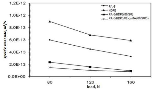
Fig. 5 - Variation of the wear rate at applied load for pure PA 6, pure HDPE, PA 6/HDPE(80/20), PA 6/HDPE/PE-g-MA(80/20/5) nanocomposites tested against stainless steel (velocity: 1 m/s).
