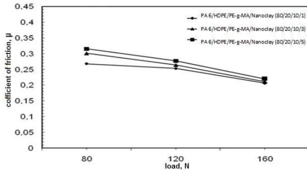
Fig. 4 - Variation of coefficient of friction at applied load for PA 6/HDPE/C/NC (80/20/10/1), PA 6/HDPE/C/NC (80/20/10/3), PA6/HDPE/C/NC(80/20/10/5) composites tested against stainless steel (velocity: 1 m/s).
