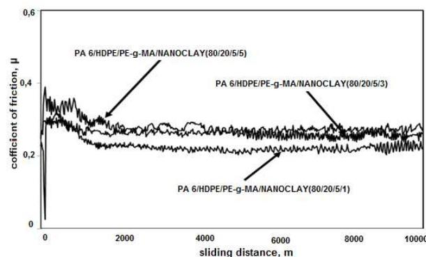
Fig. 9 - Coefficient of friction-sliding distance graph of PA 6/HDPE/PE-g-MA/Nanoclay (80/20/5/1), PA 6/HDPE/PE-g-MA/Nanoclay (80/20/5/3), PA 6/HDPE/PE-g-MA/Nanoclay (80/20/5/5) materials (load: 80 N, sliding speed: 1 m/s).
