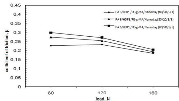
Fig. 3 - Variation of the coefficient of friction at applied load for PA 6/HDPE/C/NC (80/20/5/1), PA 6/HDPE/C/NC (80/20/5/3), PA 6/HDPE/C/NC(80/20/5/5) composites tested against stainless steel (velocity: 1 m/s).
