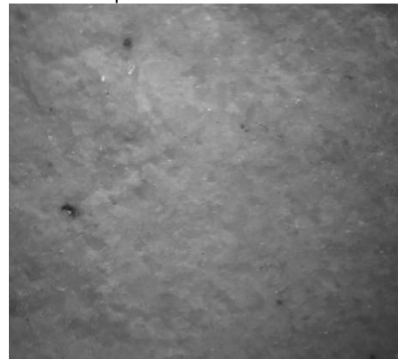
Fig. 9 - Concrete sample K2 recorded at 1400°C.
